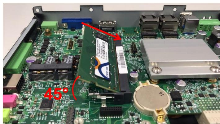
3. Press the modules down until it's fixed firmly by the two locking latches on each side.
