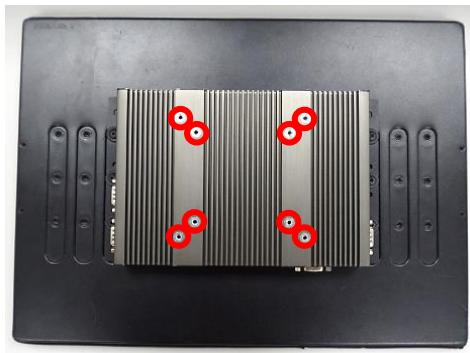
2. Put on the rack mount base and fasten the screws.
