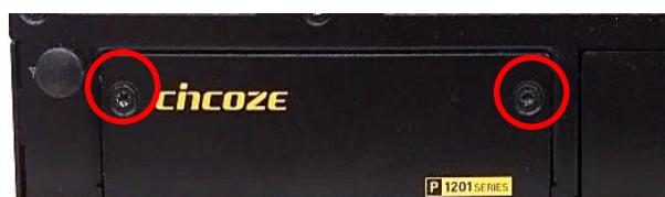
4. IGN function switch is at the front panel of the system.
