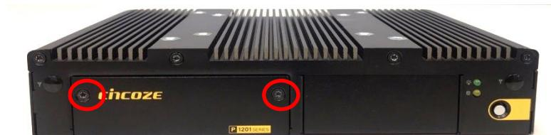
2. SIM card slot is at the front panel of the system.
