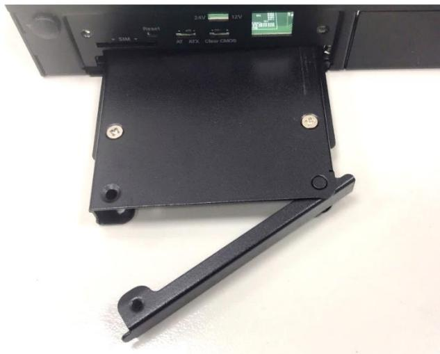
6. Turn over the unit to have the bottom side face up and fasten the screw.
