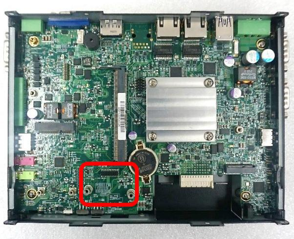
2. Insert CFM-IGN module vertically to the female connector on the system's mainboard, and fasten 2 screws to fix it.
