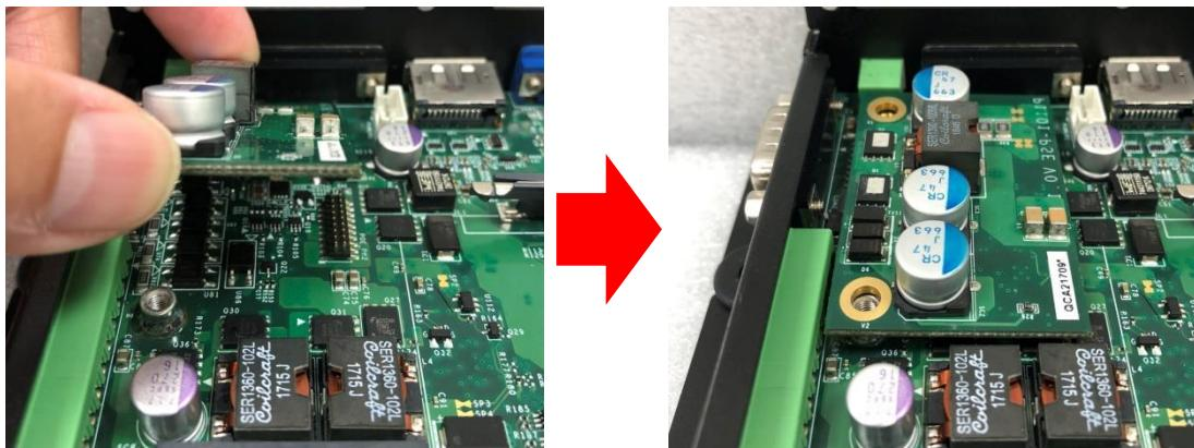
3. Turn over the heatsink and paste the thermal pad onto the marked by red squares.
