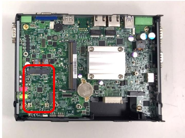
2. Insert the Mini-PCIe card at a 45-degree angle and insert it to the slot until the gold-pated connector of module contacted firmly with the slot.
