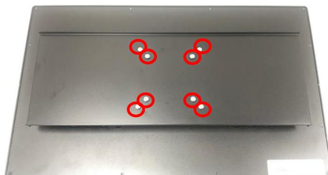
3. Locate the Rack mount bracket holes.
