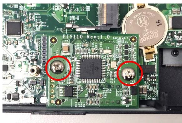
3. Loosen 2 screws on front panel to remove cover plate.
