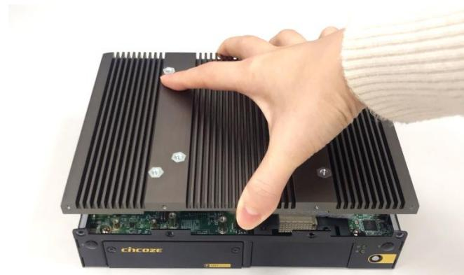
2. Fasten the 8 screws to fix the cover.
