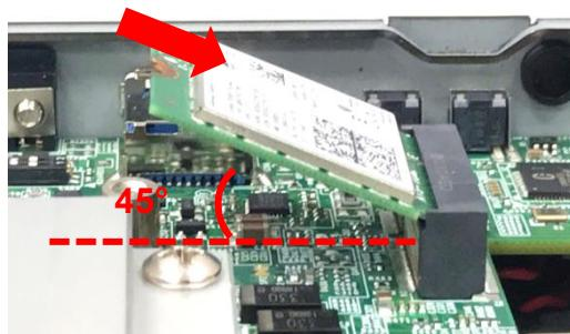
3. Press the card down and secure it with 1 screw.
