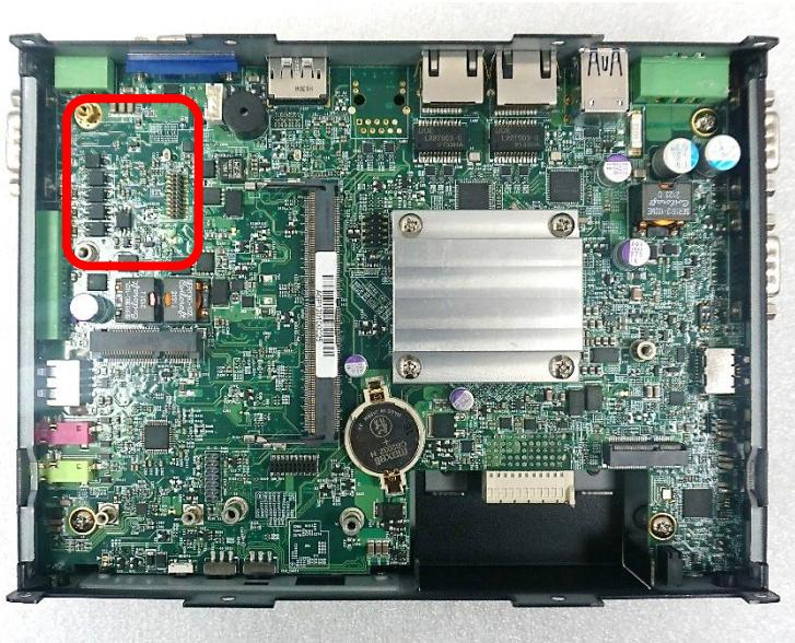
2. Insert the female connector of CFM-PoE module to the male connector on system motherboard.
