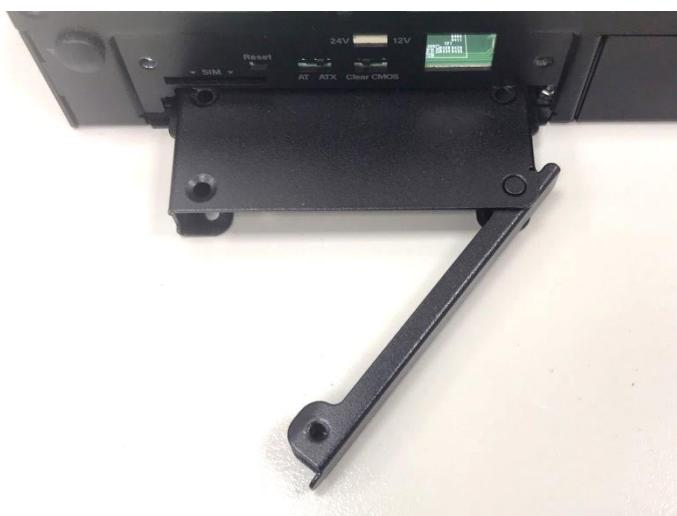
4. Make the bottom side of the HDD face up, place the HDD bracket on it. Ensure the direction of bracket is correct and use 4 provided screws to assemble HDD and HDD bracket together.
