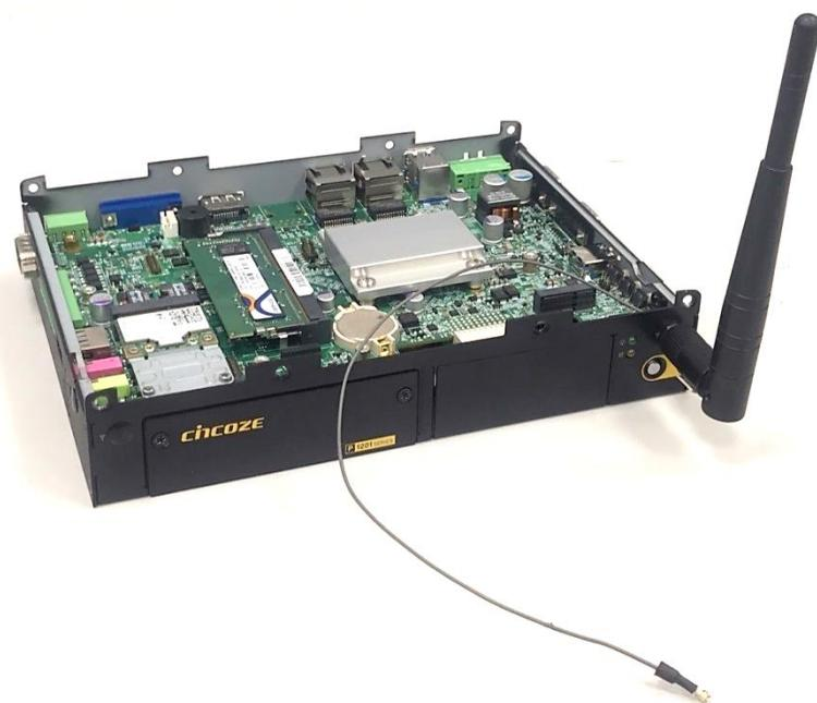
5. Attach the RF connector at another end of cable onto the module.
