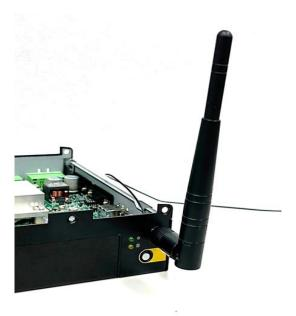
Step 5. Attach the RF connector at another end of cable onto the module.
