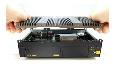
Step2. Fasten the 8 screws to fix the cover.
