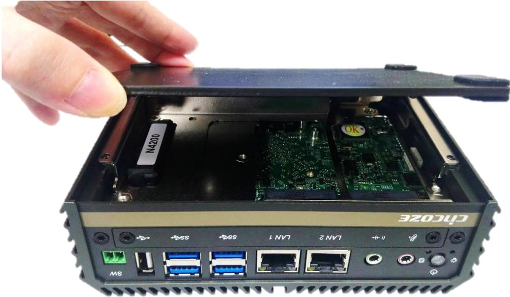
3. Fasten the 4 screws to fix the cover.
