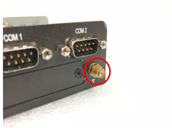
4. Assemble the antenna and antenna jack together.
