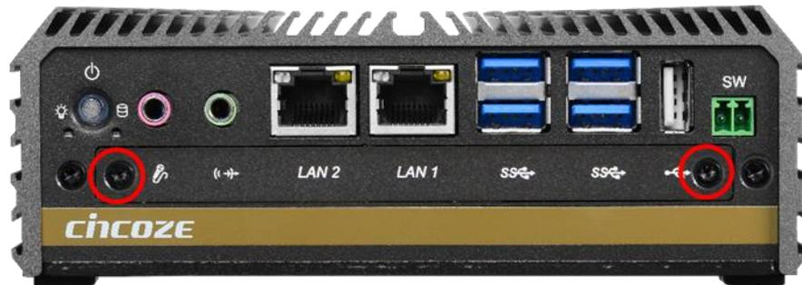
2. SIM card slots are at the front panel of the system.
