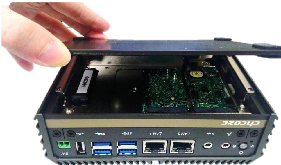
3. Hold front and rear panel and lift up the body of unit vertically.
