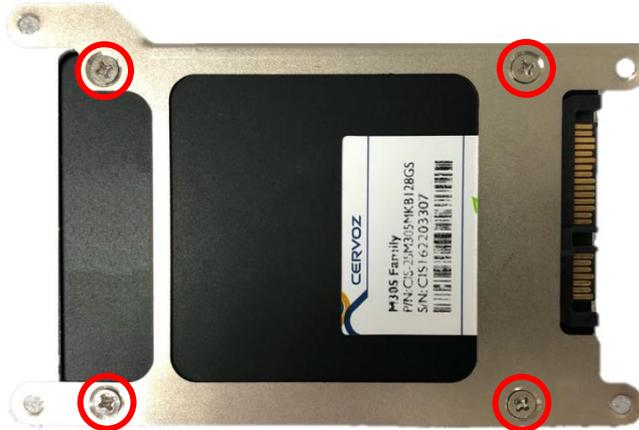
3. Turn over the HDD bracket. Connect the HDD bracket to the SATA connector of the unit and fasten the 3 screws.
