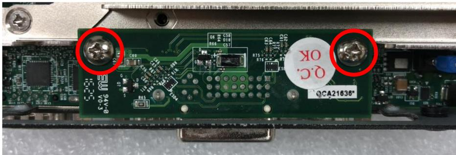
3. Attach the CMI-DVI bracket, and fasten 2 screws as marked on photo.
