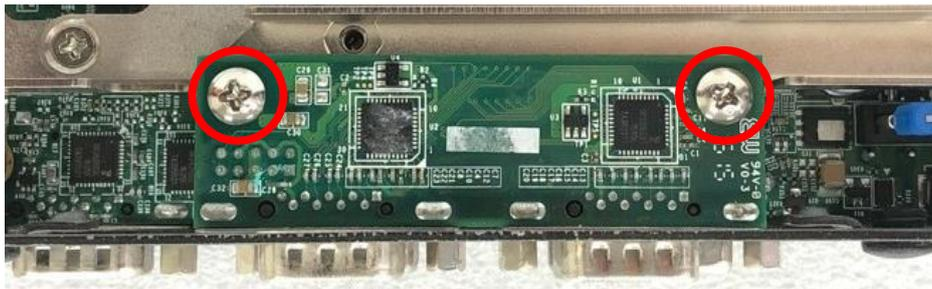
3. Attach the CMI-COM bracket, and fasten 2 screws as marked on photo.
