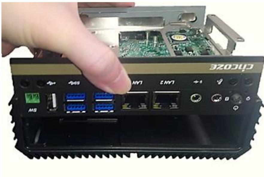
2. Level the grooves on the cover at front and rear panels. Put on the cover.
