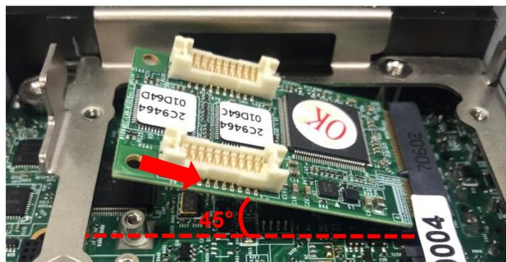
5. Press the card down and secure it with 2 screws.
