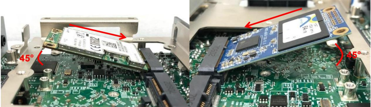
4. Press down the module and fasten two screws to secure the module.
