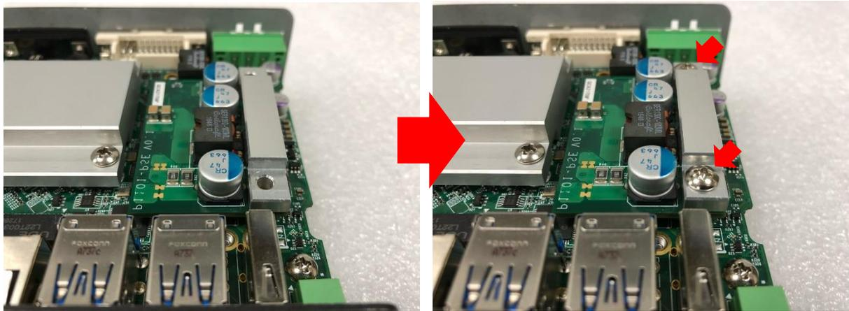
5. Paste the thermal pads onto the heatsink and coil carefully.
