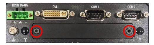
2. Insert CMI-HD module vertically to the female connector on the system's mainboard, and fasten 2 screws to fix it.
