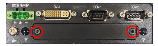
2. Insert CMI-LPPS module vertically to the female connector on the system's mainboard, and fasten 2 screws to fix it.
