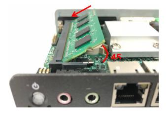
3. Press the modules down until it's fixed firmly by the two locking latches on the sides.
