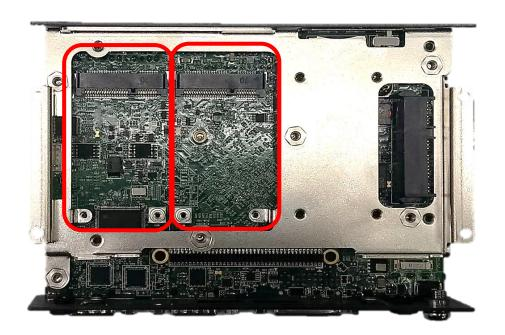
3. Insert the Mini-PCIe card at a 45-degree angle and insert it to the slot until the gold-pated connector of module contacted firmly with the slot.
