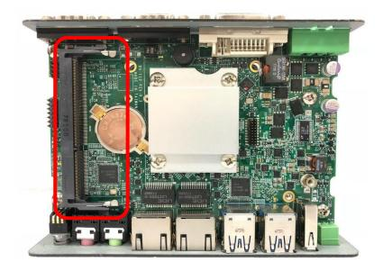
2. Tilt the SO-DIMM module at a 45-degree angle and insert it to SO-DIMM socket until the gold-pated connector of module contacted firmly with the socket.
