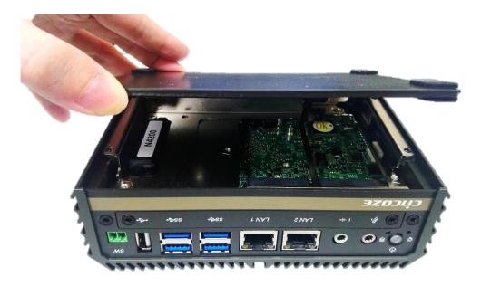
3. Hold front and rear panel and lift up the body of unit vertically.
