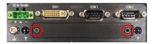
2. Insert CMI-DIO module vertically to the female connector on the system's mainboard, and fasten 2 screws to fix it.
