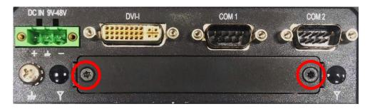
2. Insert CMI-VGA module vertically to the female connector on the system's mainboard, and fasten 2 screws to fix it.
