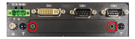
2. Insert CMI-COM module vertically to the female connector on the system's mainboard, and fasten 2 screws to fix it.
