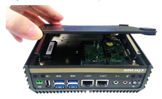
3. Fasten the 4 screws to fix the cover.
