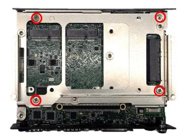
2. Make the PCB side of the HDD face up, place the HDD bracket on it. Ensure the direction of bracket is correct and use 4 provided screws to assemble HDD and HDD bracket together.
