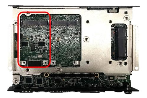
4. Tilt the Mini PCIe card at a 45-degree angle and insert it to the socket until the golden finger connector of the card seated firmly.
