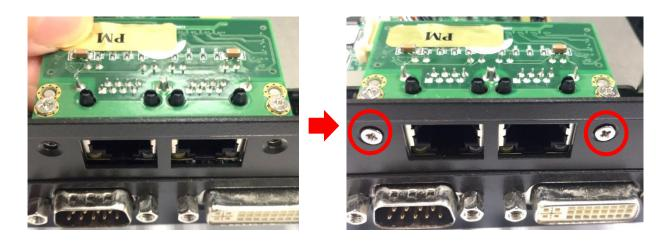
8. Connect the other end of the wire to the Mini PCle board as indicated.
