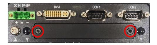
2. Insert CMI-DP module vertically to the female connector on the system's mainboard, and fasten 2 screws to fix it.
