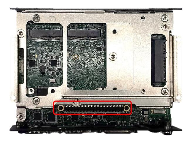
Locate the CMI connector on system motherboard as indicated.
