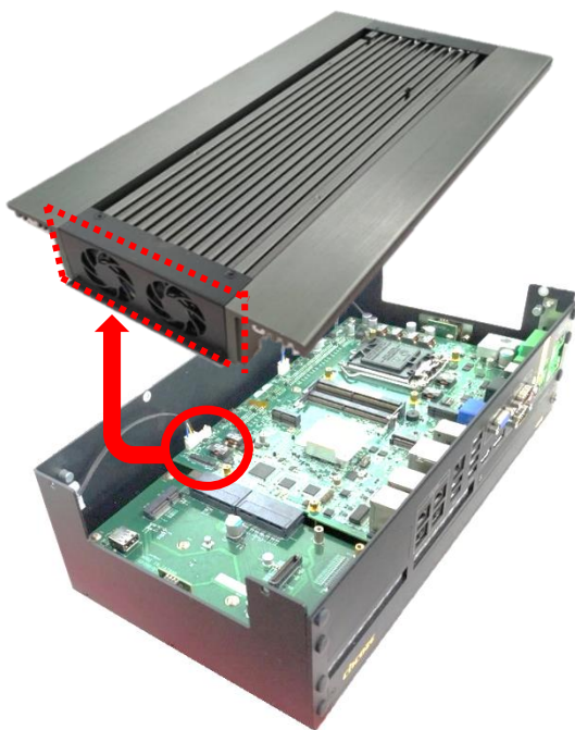
POWER1 (FAN OUT Control)
