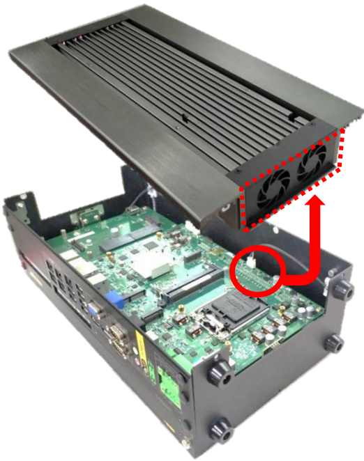
POWER2 (FAN IN Control)
