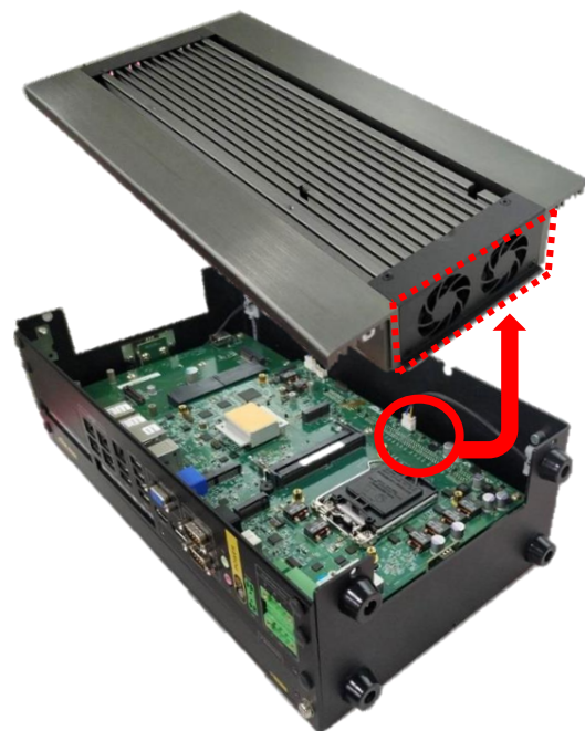
POWER2 (FAN IN Control)
