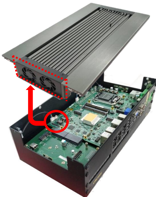
POWER1 (FAN OUT Control)
