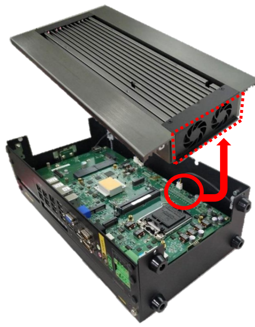
POWER2 (FAN IN Control)
