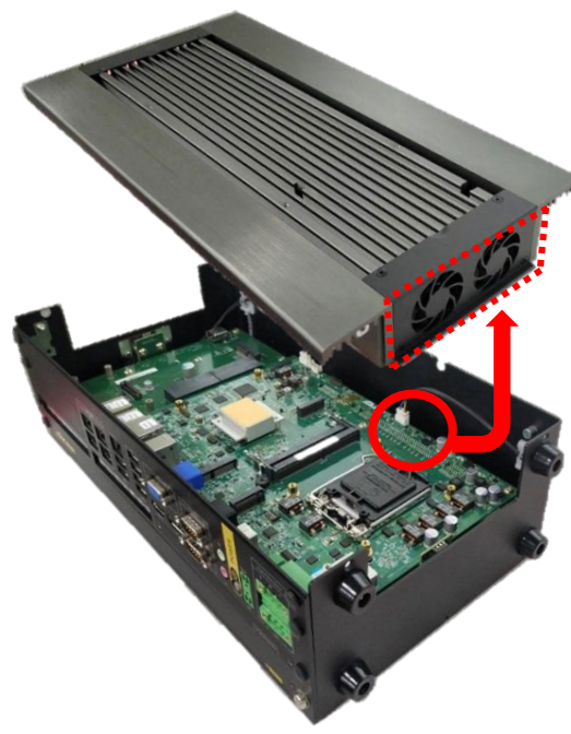
POWER2 (FAN IN Control)
