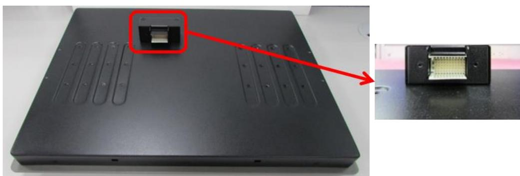
6. Place the P2102 on the display module through its display connector hole as indicated.
