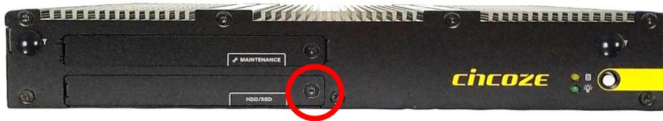
8. Fasten the screw to secure the HDD bracket on the system chassis.
