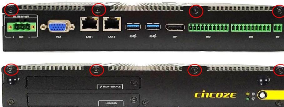
2. Raise the edge of top cover (1), and raise the other side (2) subsequently to remove it from the chassis.
