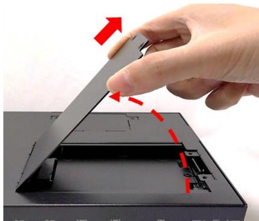
3. Loosen three screws and take the HDD bracket out of HDD compartment.
