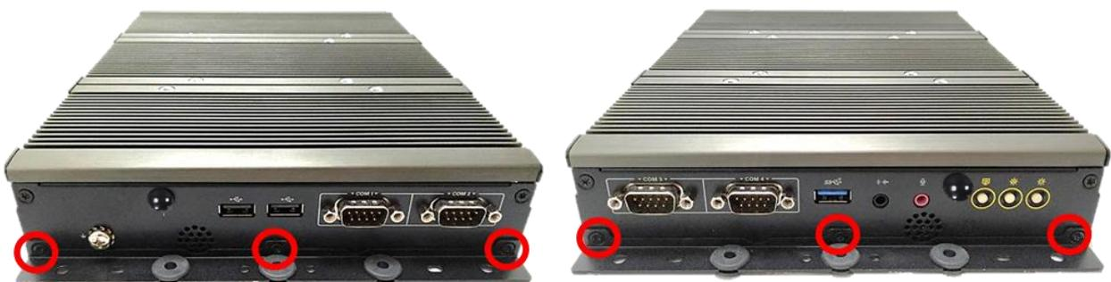
The following picture indicates six wall mounting holes at each side.
