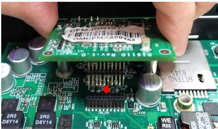
3. Fasten two screws to secure the power ignition board.
