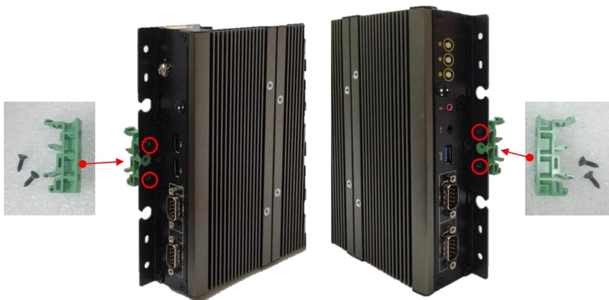
3. Clip the system into DIN rail as illustrated by the following steps. (1) Have lower end of mounting clip snaps into the DIN rail. (2) Press the system toward to have upper end of mounting clip snaps into the other side of DIN rail.
