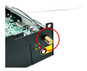
Step 3. Put on the washer and fasten the nut with the antenna jack.
