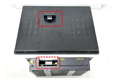
Step 4. Align the two connectors to connect them together as illustrated below.
