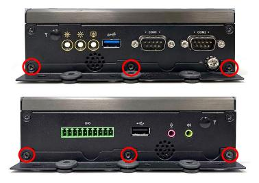
Step 4. Attach the system to the wall by fastening four screws through the mounting holes at each side as illustrated.
