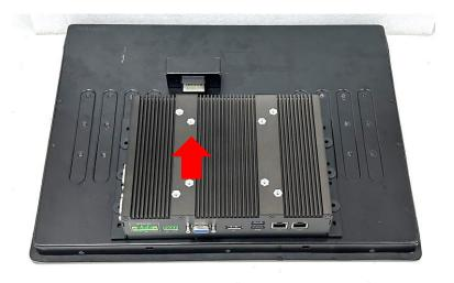
Step 5. Fasten the 6 screws to fix the system on the display module.
