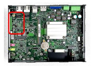
Step 2. Insert the female connector of CFM-PoE module to the male connector on system motherboard.
