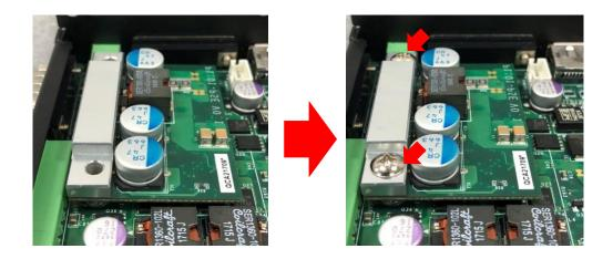
Step 5. Paste the thermal pads onto the heatsink and coil carefully.
