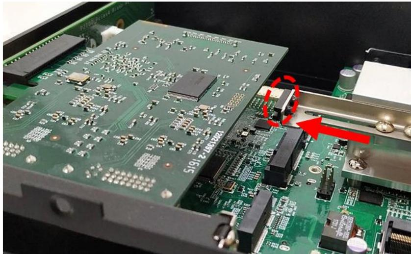
10. Finally, fasten the two screws that were previously loosen halfway to fix the retention module.
