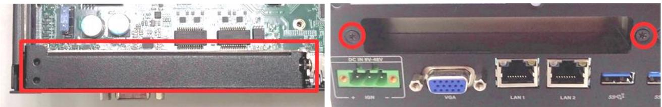
3. Loosen the screw as indicated to remove the PCI bracket.
