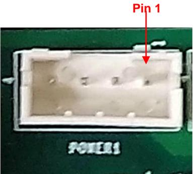
**PWR\_SW1: Remote Power On/Off Switch Connector**
