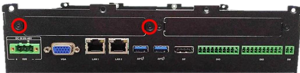
2. Attach the PCI / PCIe Card Installation Kit on, and fasten the two screws back on rear panel to fix the Kit.
