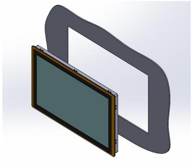
2. All mounting kits displayed are to be inserted into holes.
