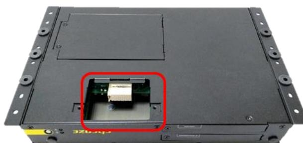
6. Place the P2102 on the display module through its display connector hole as indicated.
