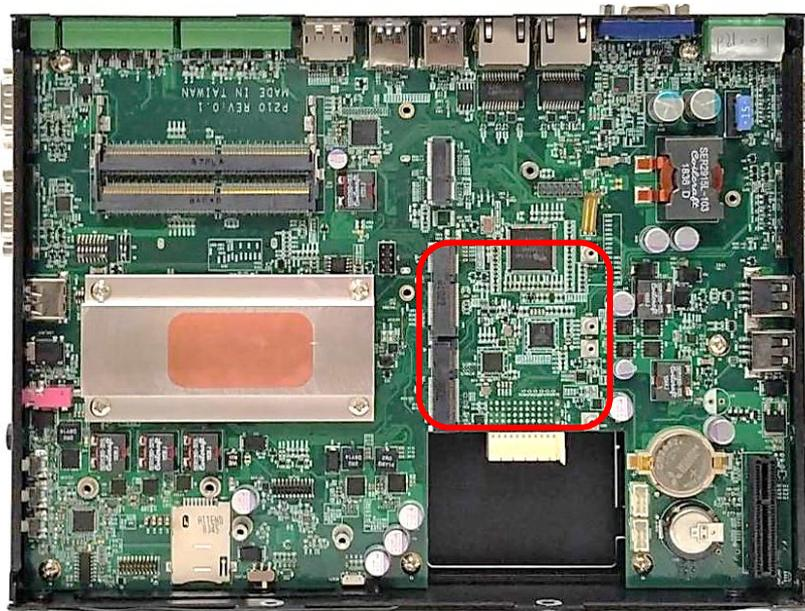
2. Tilt the Mini PCIe card at a 45-degree angle and insert it to the socket until the golden finger connector of the card seated firmly.
