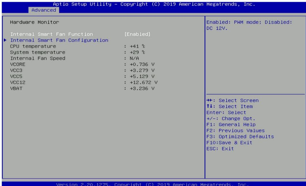
■ **Internal Smart Fan Function [Enabled]**
