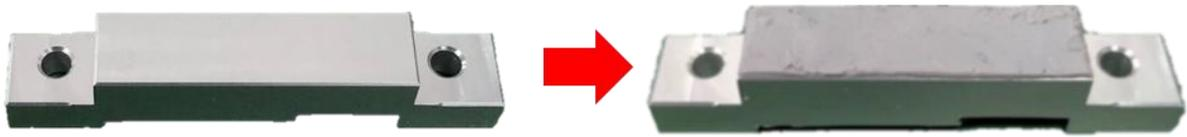
2. Turn over the heatsink and paste the thermal pad at the marked region.
