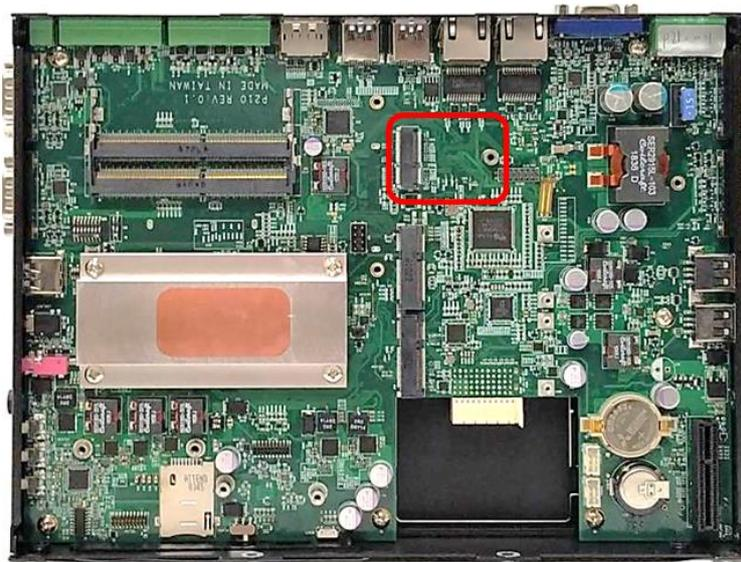
2. Tilt the M.2 E Key card at a 45-degree angle and insert it to the socket until the golden finger connector of the card seated firmly.
