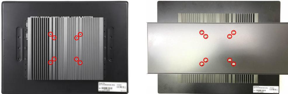
2. Assemble two rack mount brackets by fastening 4 screws (M5x6) at each side.
