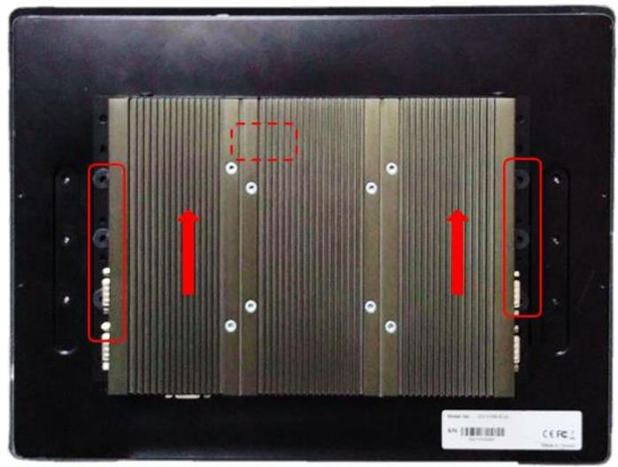
8. Fasten six screws to secure P2102 on the display module.
