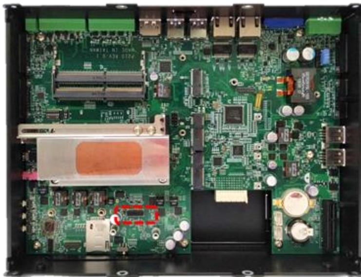
2. Insert the female connector of power ignition board to the male connector on system motherboard.
