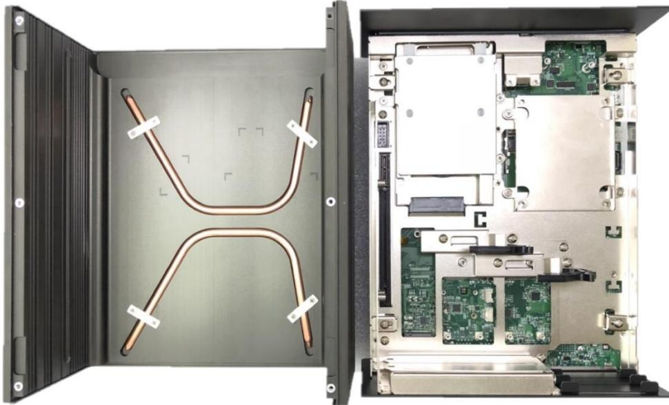
2. Lift up the body of unit. Make sure that both front and rear panels are in the chassis grooves and assemble the body on to chassis firmly.
