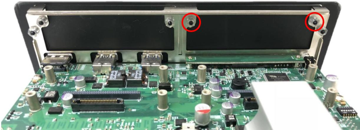
2. Locate the connector of CMI-module on the top side of system.
