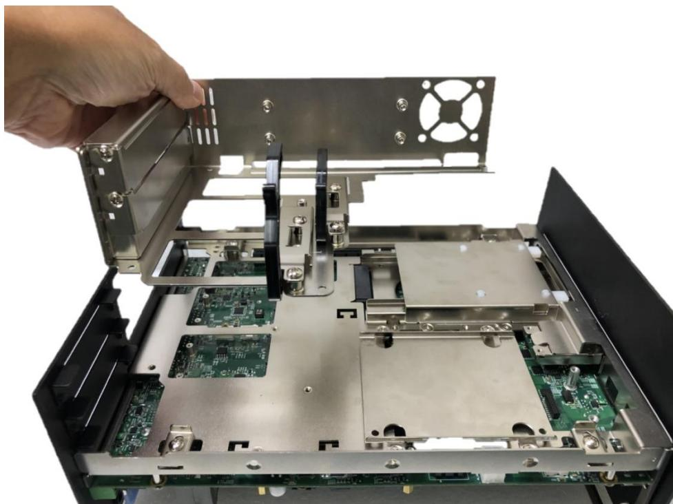
4. Assemble the riser card with extension bracket together and fasten with the 4 screws.
