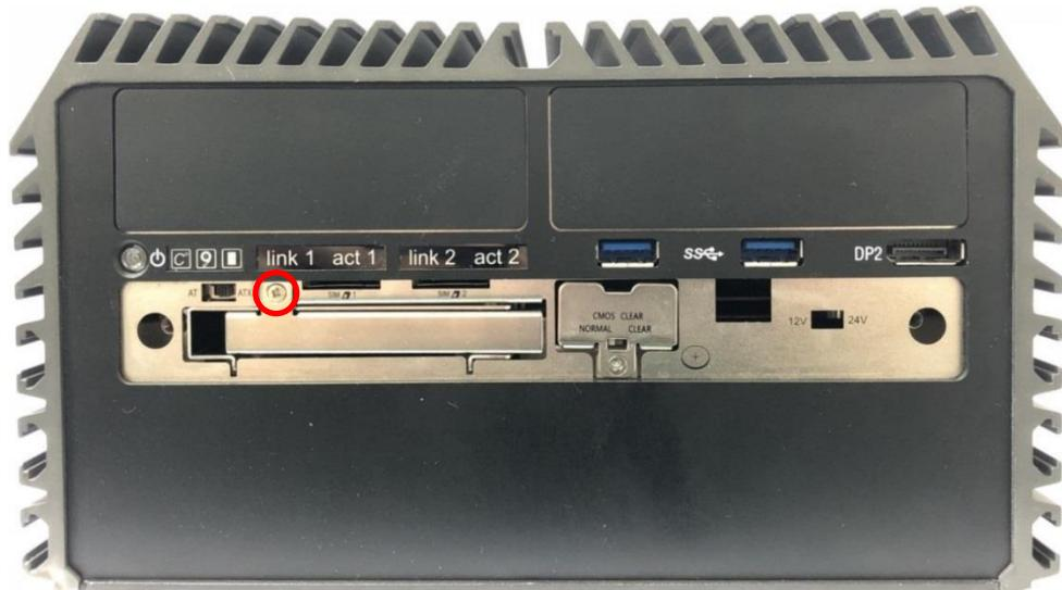
2. Move the rotating arm out and pull the HDD bracket out.
