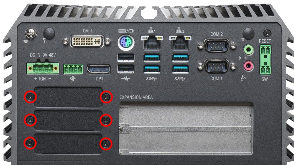
2. Attach the FAN from back side of rear panel. Fasten 4 screws to fix it.
