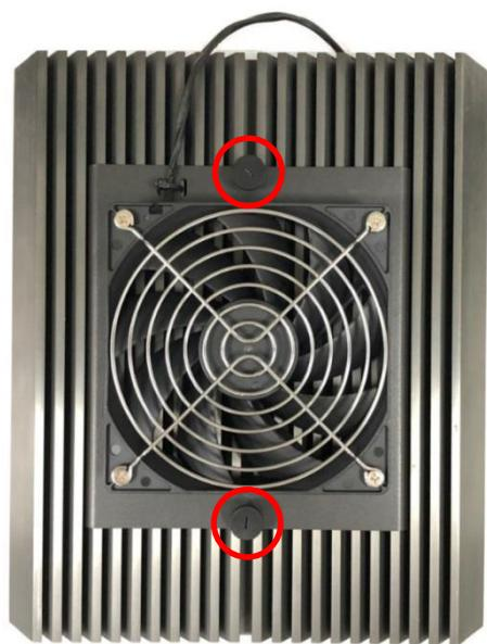
4. Connect the FAN cable to external fan power connector at rear panel.
