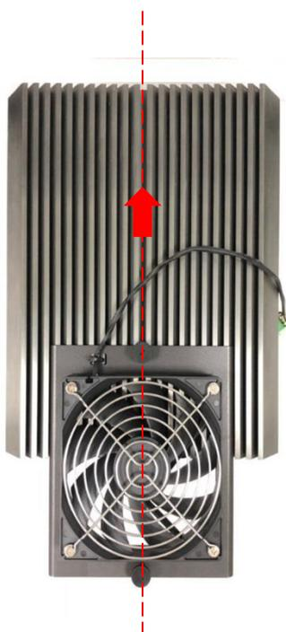
3. Move the fan to the center of chassis. Tighten the 2 screws marked on photo to secure it.
