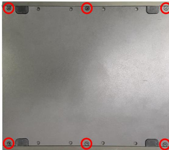
2. Remove the bottom cover from the chassis.
