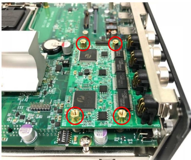
2. Insert the CFM-PoE module vertically into the female connector on CMI module until it's connected firmly.
