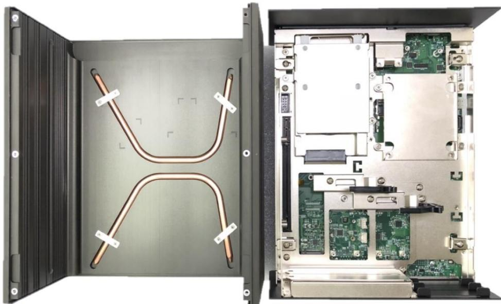
2. Lift up the body of unit. Make sure that both front and rear panels are in the chassis groves and assemble the body on to chassis firmly.
