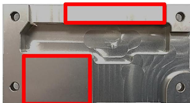
4. Please paste the 2 thermal pads onto the heatsink carefully.
