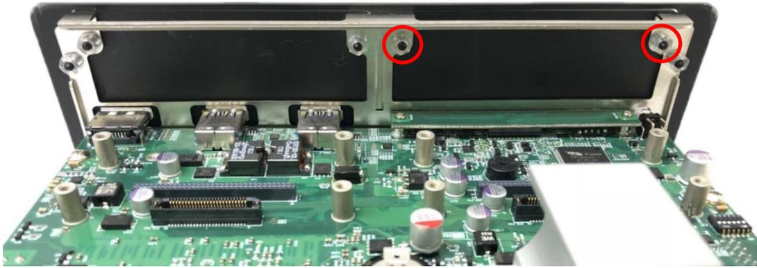
3. Locate the connector of CMI module on top side of system.
