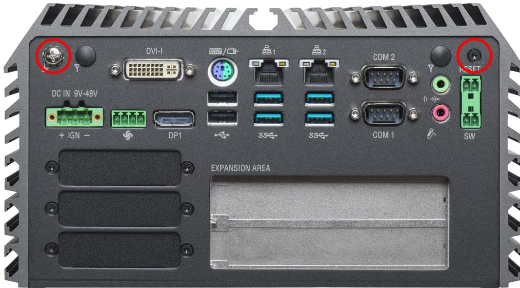
4. Loosen the 4 screws. Pull out 4 latches as marked on the photo.
