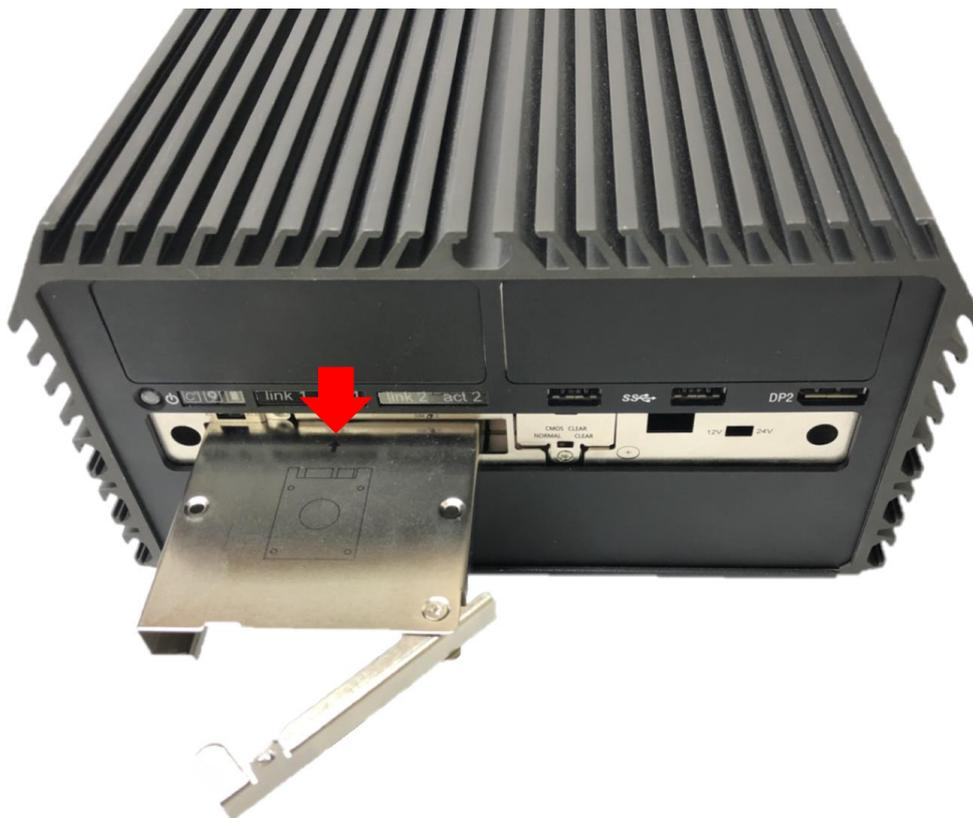
3. Make the PCB side of the HDD face up, place the HDD bracket into it. Ensure the direction of bracket is correct and use 4 provided screws to assemble HDD and HDD bracket together.
