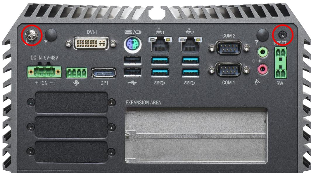
5. Be sure to align the grooves with front and rear panels. Put the cover back on and fasten the 6 screws to fix the cover.
