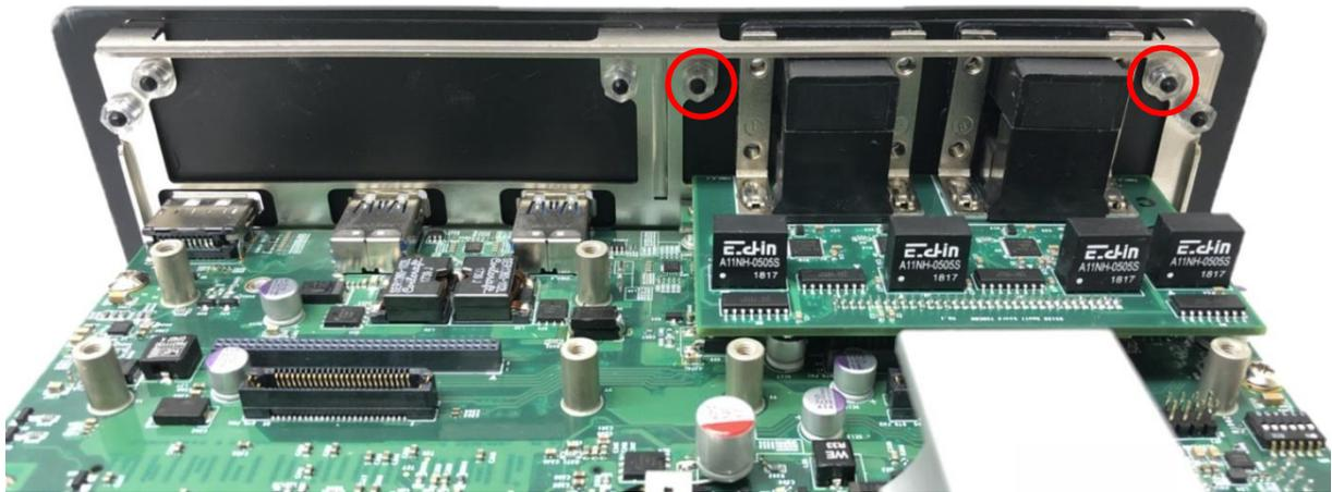
5. Fasten the 8 D-Sub jack screws as marked on photo.
