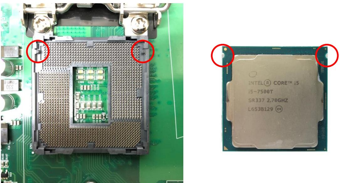
4. The notches of socket provide the space for fingers while lowering the CPU, hold the CPU by the edges toward the notches and insert the CPU gently.
