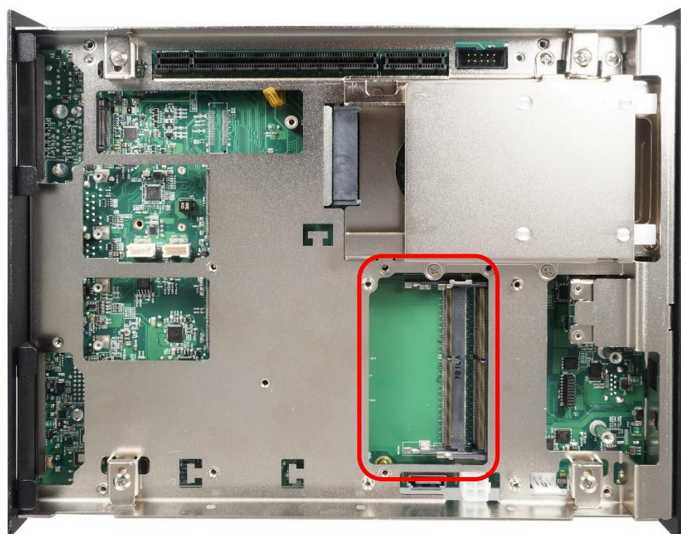
3. Tilt the SO-DIMM module at a 45-degree angle and insert it to SO-DIMM socket until the gold-pated connector of module contacted firmly with the socket.
