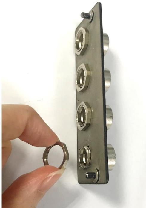
2. Loosen the 2 hex nuts from back side of front bezel. Remove the front bezel.
