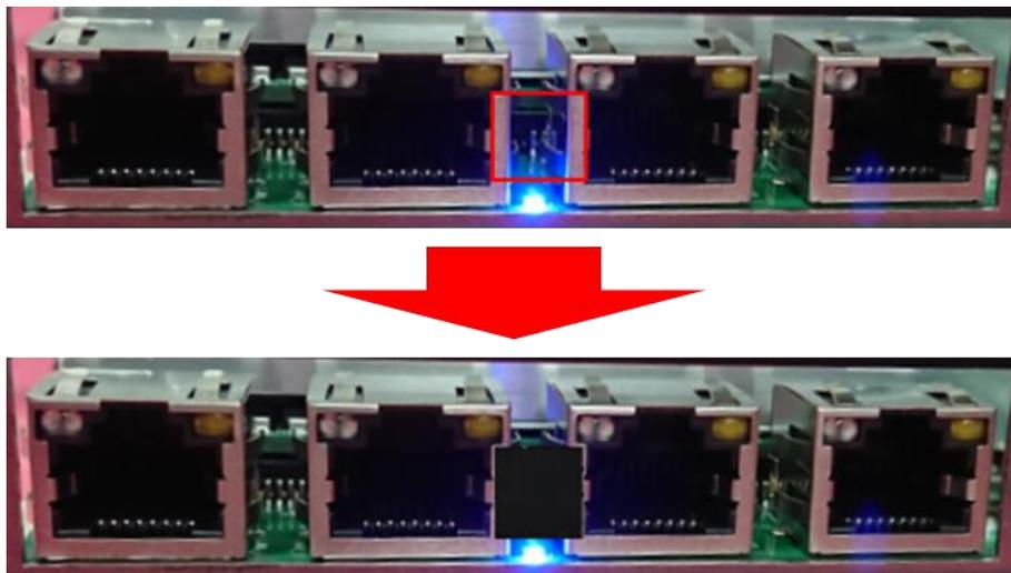
1. Insert the CMI module vertically into the female connector on system's mainboard until it's connected firmly and fasten 4 copper pillars to fix it.
