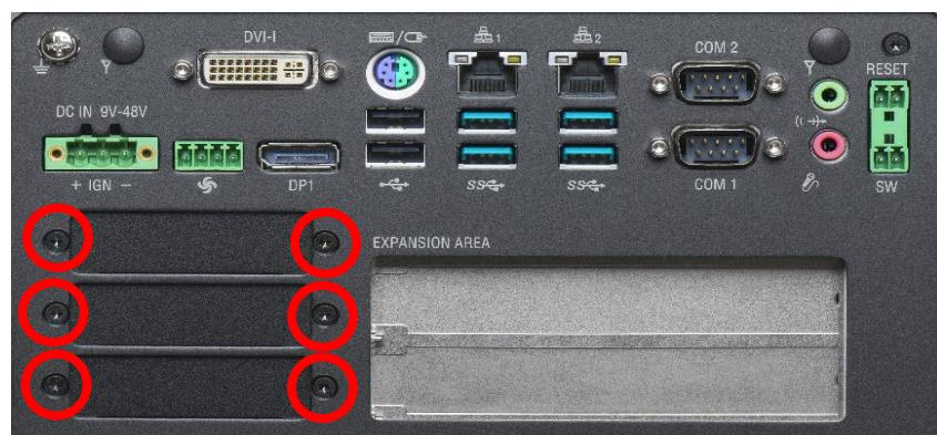
2. Attach the I/O bracket on to the system as indicated below, and fasten the screws back to fix it. For guidance on antenna installation methods, please refer to chapter 3.6.
