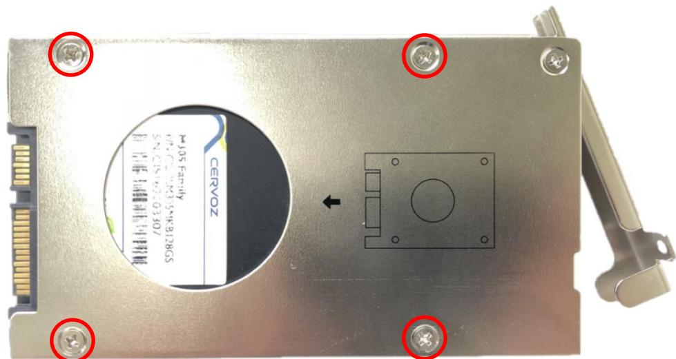
4. Align the HDD bracket with the entrance of HDD bay. Holding the rotating arm and insert the HDD bracket until the connector of HDD contact the SATA connector firmly.
