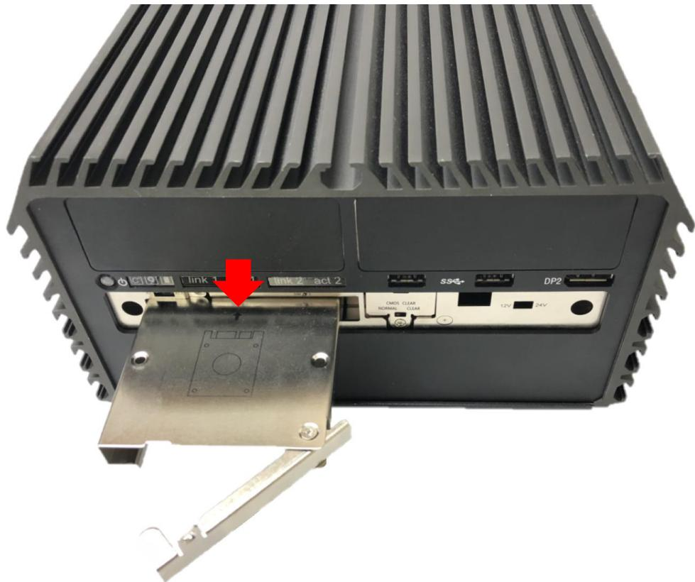
3. Make the PCB side of the HDD face up, place the HDD bracket into it. Ensure the direction of bracket is correct and use 4 provided screws to assemble HDD and HDD bracket together.
