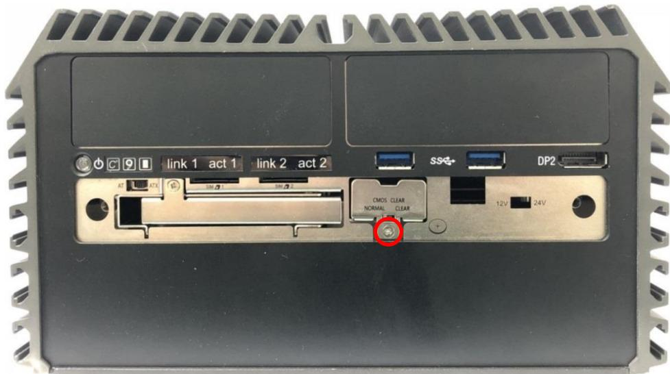
2. Pull out the CMOS battery bracket with assistance of a tweezer.
