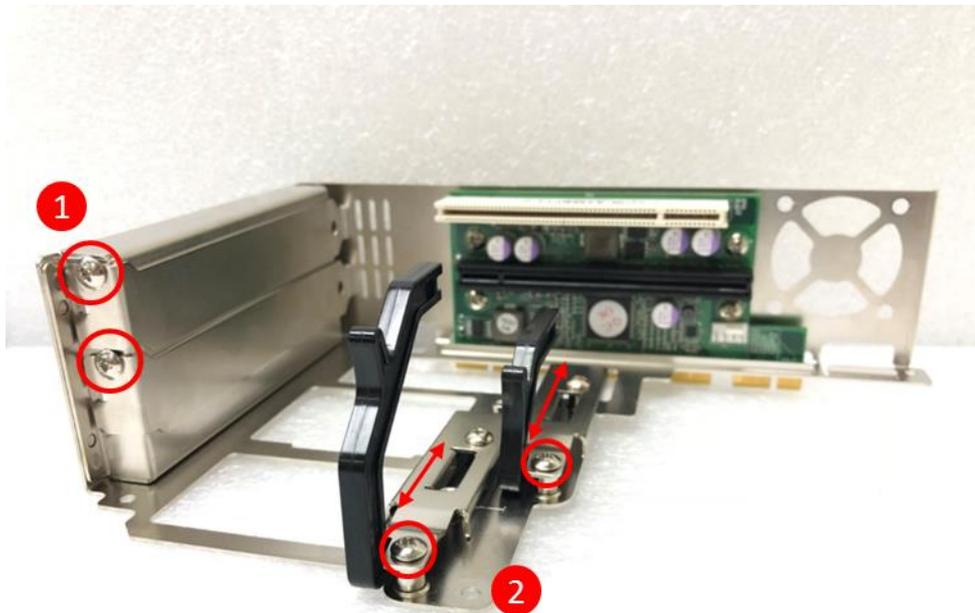
6. (1) Insert a PCI(e) add-on card to the slot. (2) Fasten the screw to secure it (3) Push the card retainer forward to against the edge of the add-on card. (4) Tighten the screw to fix the card retainer.
