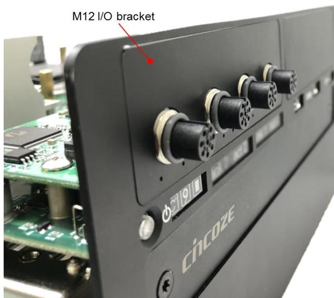
6. Fasten 2 hex nuts from the back side of the bracket.
