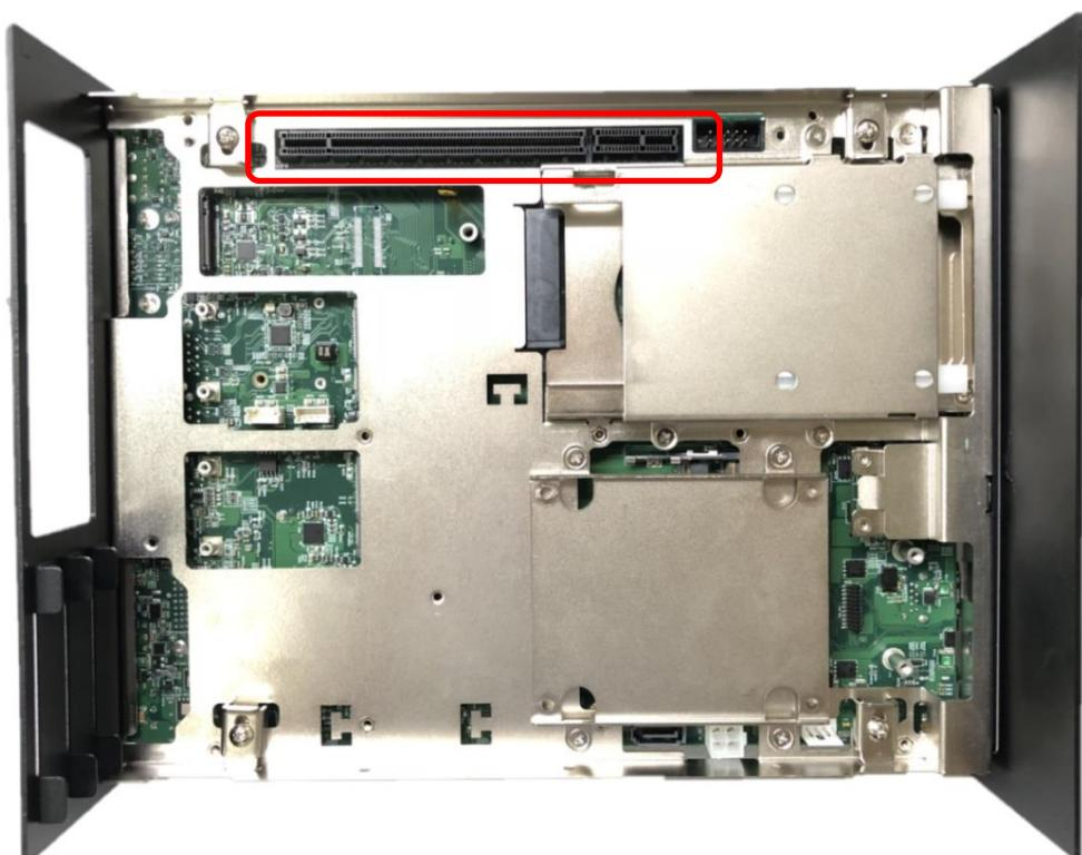
8. Install the module assembled in step 4 into the riser card slot, and fasten the 4 screws to secure it.
