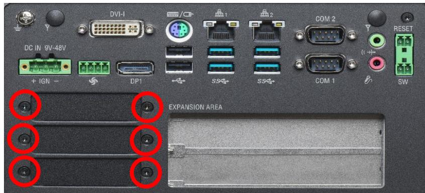
2. Attach the I/O bracket on to the system as indicated below, and fasten the screws back to fix it. For guidance on antenna installation methods, please refer to chapter 3.6.
