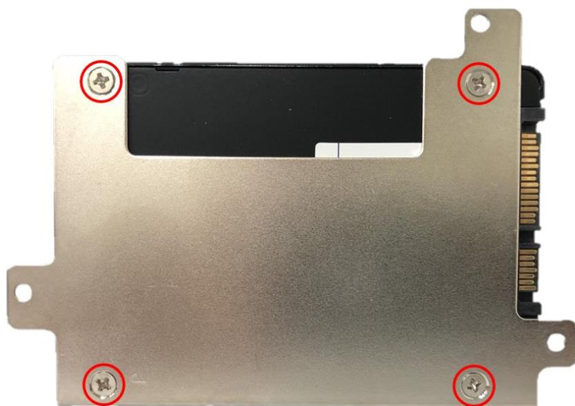
3. Turn over the HDD bracket. Connect the HDD bracket to the SATA connector and fasten the 3 screws.
