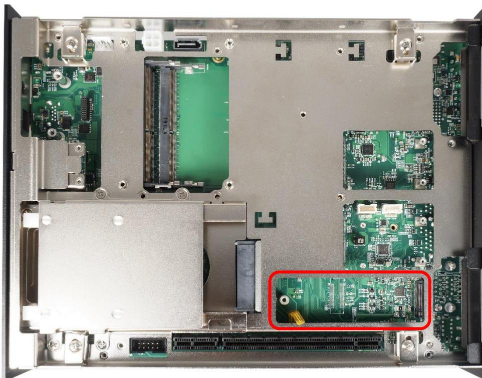
3. Tilt the M.2 M Key card at a 45-degree angle and insert it to the slot until the gold-pated connector of module contacted firmly with the slot.
