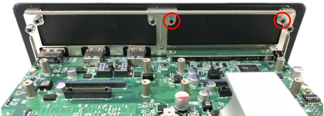
2. Locate the connector of CMI module on top side of system.
