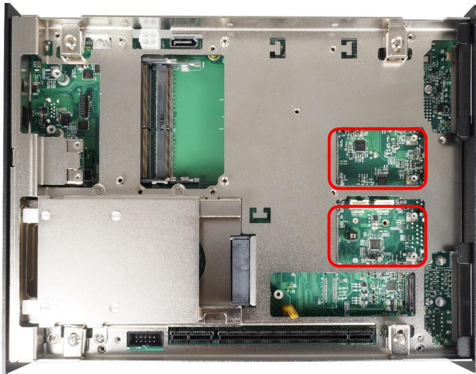
2. Tilt the Mini-PCIe module at a 45-degree angle and insert it to the slot until the gold-pated connector of module contacted firmly with the slot.
