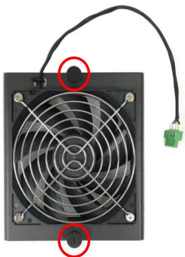
2. Slide the FAN into the middle groove of chassis as illustrated. Tighten the 2 screws to fix it onto chassis.
