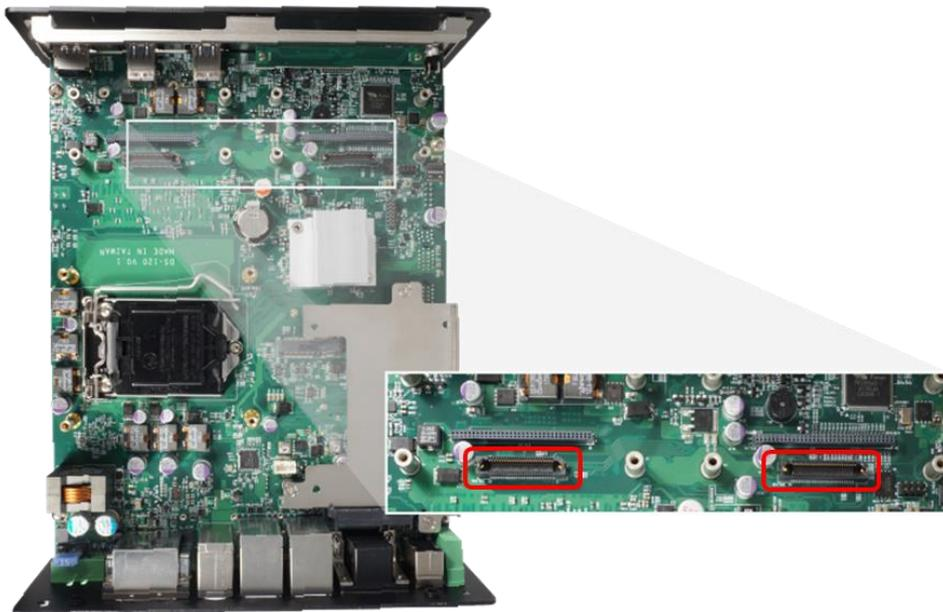
4. Insert the CMI module vertically into the female connector on system's mainboard until it's connected firmly and fasten 4 screws to fix it.
