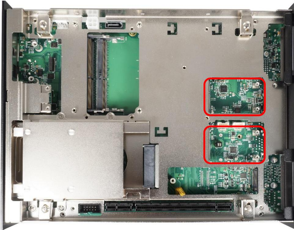
2. Tilt the Mini-PCle module at a 45-degree angle and insert it to the slot until the gold-pated connector of module contacted firmly with the slot.
