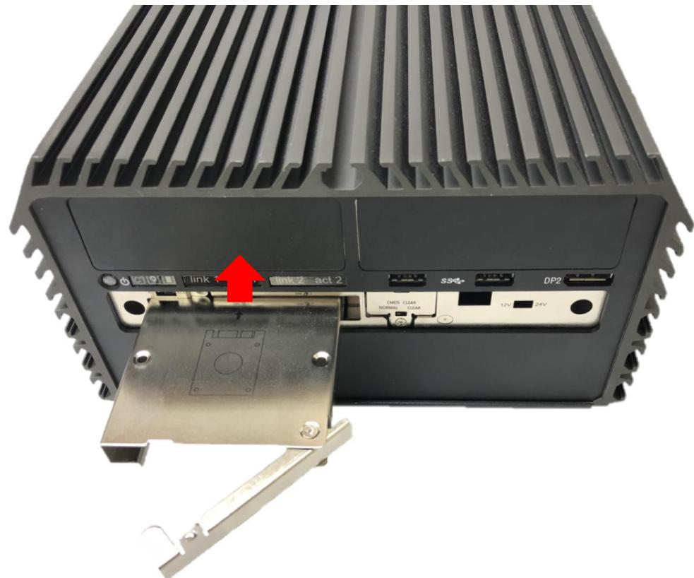
5. Place the rotating arm back and fasten the screw.
