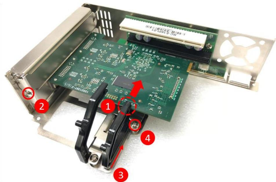
7. Locate the riser card slot on bottom side of system.
