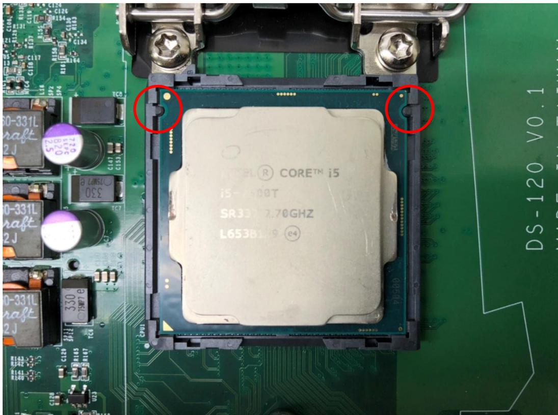
5. Place the thermal pad on the CPU heat spreader. Press down the socket lever to lock the CPU.
