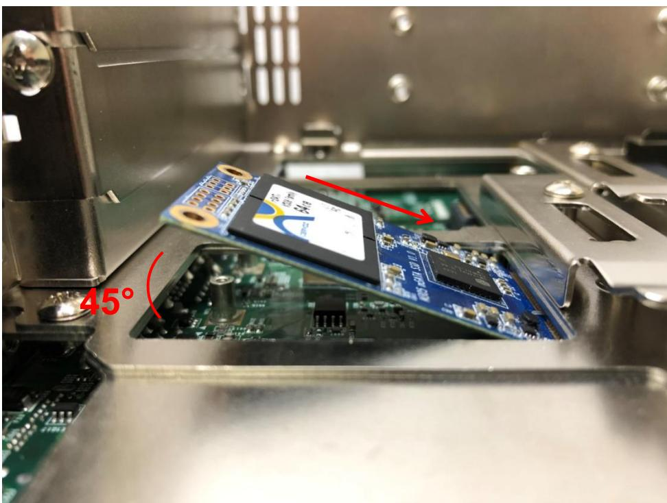
3. Press down the module and use previous two screws to fix the module.
