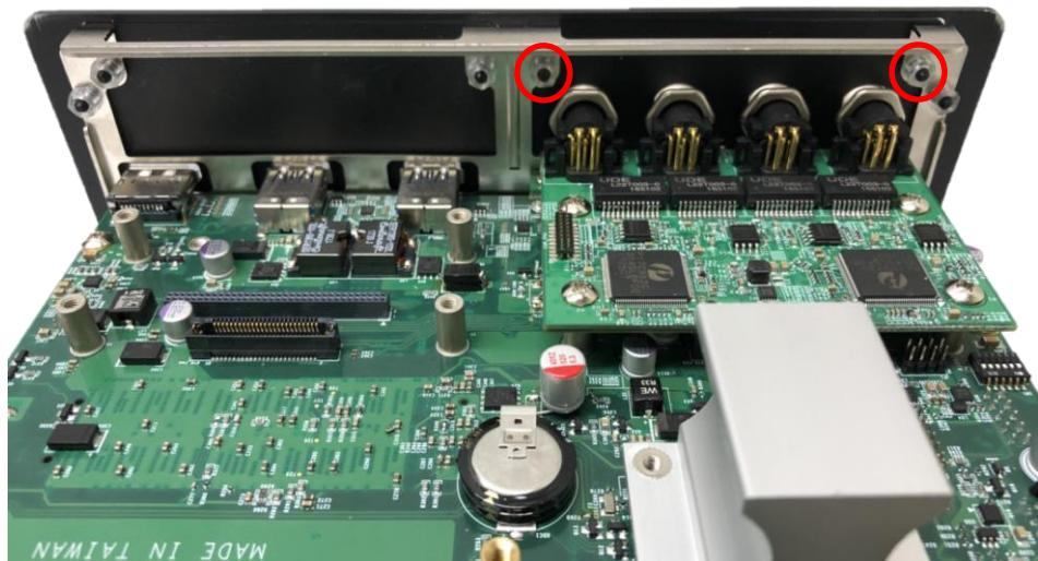
7. Fasten the 4 ring nuts onto M12 jacks.
