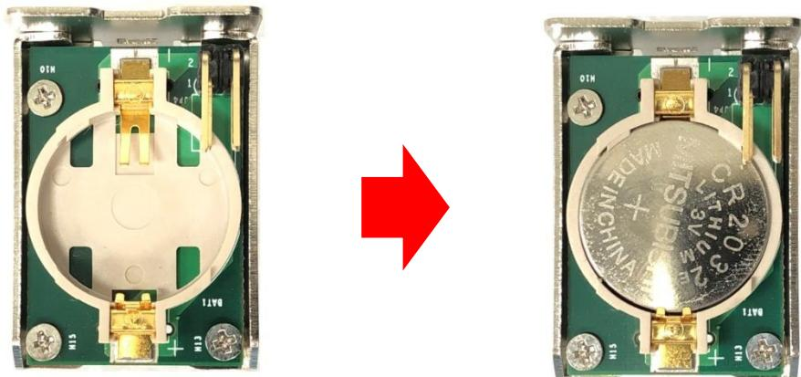
4. Insert the battery bracket firmly and fasten the screw.
