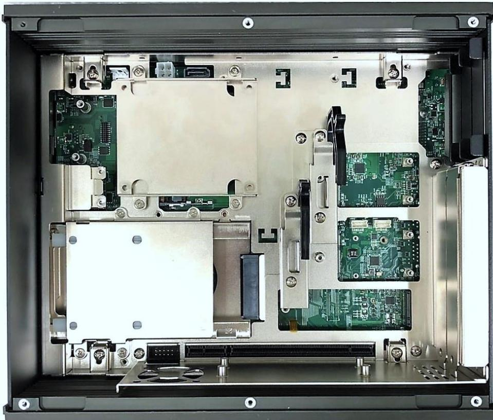
3. Push into the 4 latches as indicated and fasten the 4 screws.
