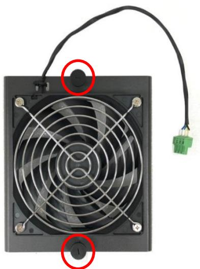
2. Slide the FAN into the middle groove of chassis as illustrated. Tighten the 2 screws to fix it onto chassis.
