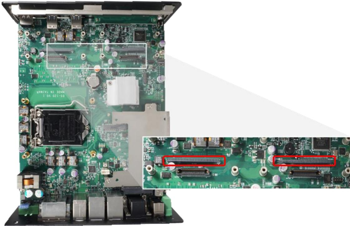
3. Insert the CMI module carefully into the CMI connector on the main board. Fix it with 4 screws.
