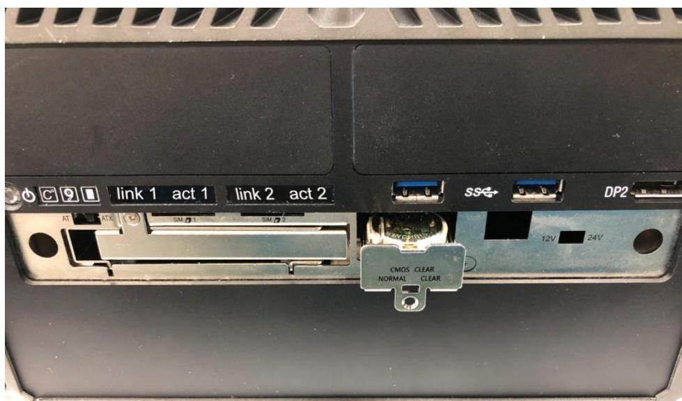
3. Insert a CMOS battery in the battery slot.
