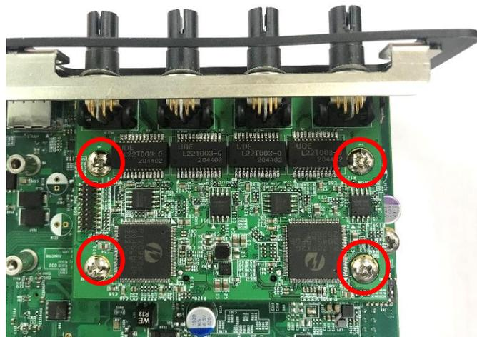
5. Attach the assembled M12 I/O bracket on to the system, and fasten the hex nuts to fix it.
