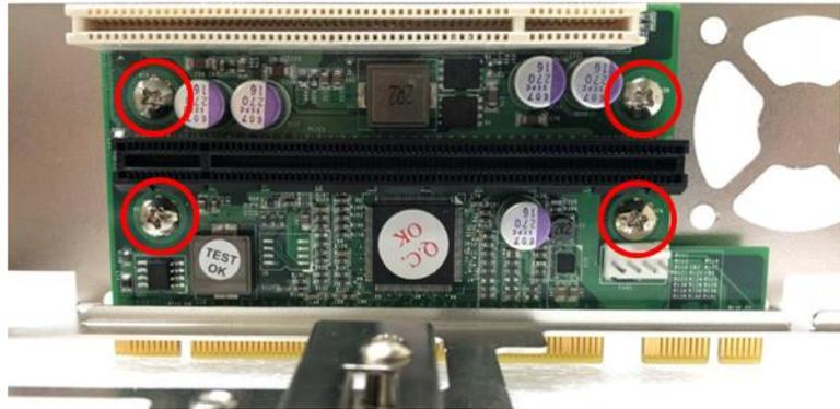
5. (1) Loosen the screw to remove I/O bracket. (2) Loosen the 2 screws halfway to allow the card retainer to be adjustable.
