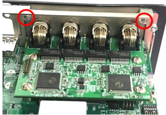
6. Put on the rubber rings to the four M12 LAN ports.
