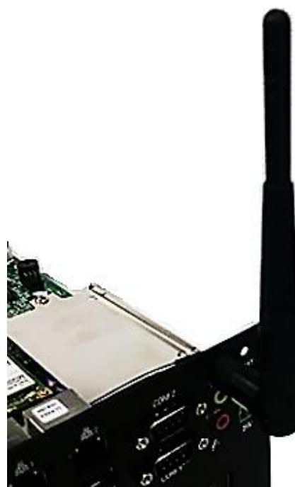
5. Attach the RF connector at another end of cable onto the module.
