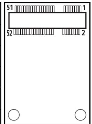
**CN8: M.2 Socket Socket (Support M.2 PCIE / SATA SSD feature)**
