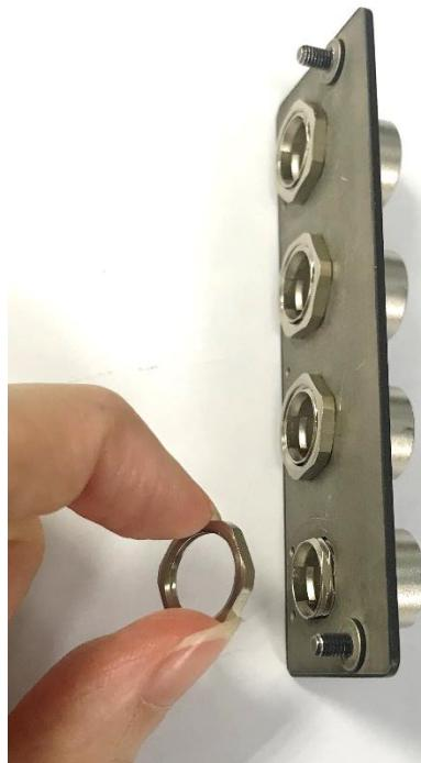
2. Loosen the 2 hex nuts from back side of front bezel. Remove the front bezel.
