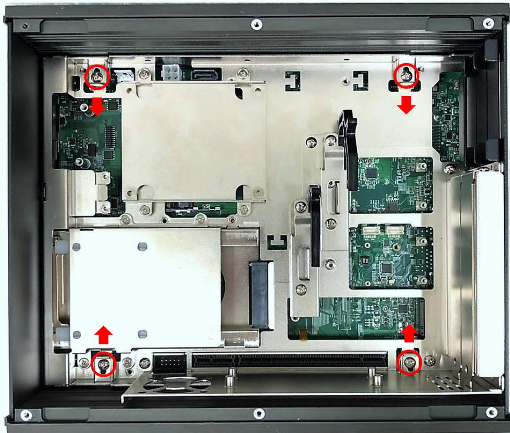
5. Lift up the unit vertically by holding the front and rear panel.
