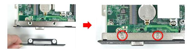
Step 6. Fasten the 2 D-Sub jack screws to fix the module. Then the installation of the module is complete.
