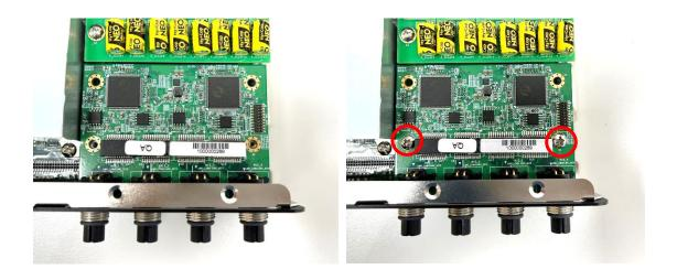
Step 5. Attach the I/O bracket on to the system, and fasten the two screws to fix it.
