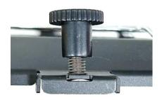
Step 3: Align the two screws and slide the fan into the middle groove of the chassis until it reaches the center position (the both screws will be in the groove at the same time).
