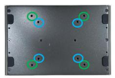
Step 1. Align the stand with the screw holes on the system, then secure it in place by tightening the corresponding number of screws as shown below. (Please note the VESA mounting holes deep 3 mm at the back of the terminal are provided with 4 x M4-type blind fasteners to fix the VESA mounting plate. A different screw length (L) should be selected.)
