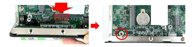
Step 4. Fasten the screw to secure it in place.
