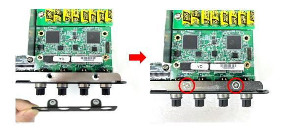
Step 6. Fasten the four hex rings back to fix the cover plate.
