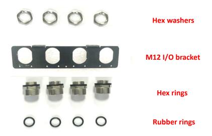
Step 1. Assemble the hex rings, M12 I/O bracket and hex washers together as indicated below: Penetrate hex rings through the M12 I/O bracket holes, and fix them with hex washers.
