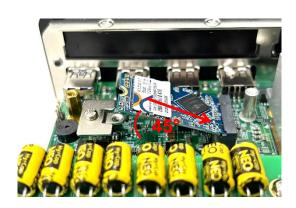
Step 4. Press down the module and fasten the screw to secure the module.
