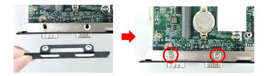
Step 6. Fasten the 4 D-Sub jack screws to fix the module. Then the installation of the module is complete.
