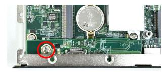
Step 5. Attach the I/O bracket on to the system, and fasten the two screws to fix it.
