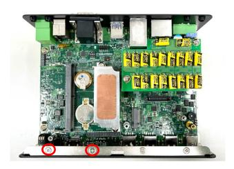
Step 3: Align the pins on the module with the connector on the right side as indicated, and then insert the CMI module vertically until it is securely connected with ensuring that the screw holes are properly aligned.
