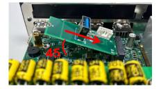
Step 3. Press down the module and fasten the screw to secure the module.
