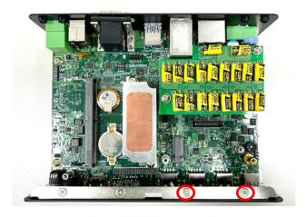
Step 3. Insert the CMI module vertically until it's connected firmly and fasten 2 screws to fix it.
