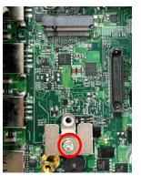
Step 3. Insert the M.2 Key B module at a 45-degree angle and insert it to the slot until the gold-pated connector of module contacted firmly with the slot.
