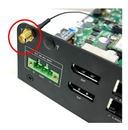
Step 4. Assemble the antenna and antenna jack together.
