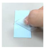
Step 2. Place the thermal pad onto the CPU heatsink, ensuring the peeled side faces downward.
