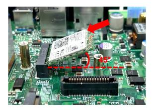
Step 3. Press the card down and secure it with one screw.
