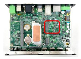
Step 3. Tilt the M.2 Key E card at a 45-degree angle and insert it to the socket until the golden finger connector of the card seated firmly.
