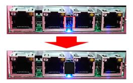
Step 1. Penetrate the copper pillars through the two holes on the LAN module, and fasten each copper pillar by the hex nut.
