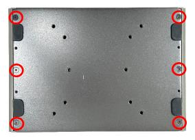
Step 2. Remove the bottom panel and then the system body from the chassis.
