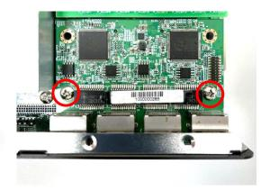
Step 4. Attach the I/O bracket on to the system, and fasten the two screws to fix it.
