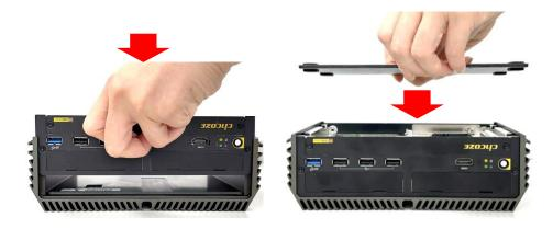
Step 2. Fasten the 6 screws back to the bottom panel of the system.
