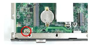
Step 5. Attach the I/O bracket on to the system, and fasten the two screws to fix it.
