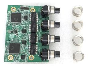
Step 4. Insert the CMI module vertically until it's connected firmly and fasten 2 screws to fix it.
