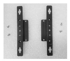
Step 1. Locate the four screw holes on the bottom panel of the system. Attach the brackets by aligning them with the four screw holes, and use the provided four screws (M3x5L) to secure the brackets on both sides of the system
