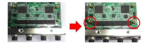
Step 3. Insert the CFM-PoE06 module vertically into the female connector on CMI module until it's connected firmly.
