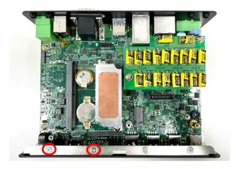
Step 3: Align the pins on the module with the connector on the left side as indicated, and then insert the CMI module vertically until it is securely connected with ensuring that the screw holes are properly aligned.
