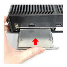
Step 6. Fasten the screw on the HDD bracket.
