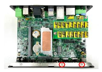
Step 4. Insert the CMI module vertically into the female connector on system's mainboard until it's connected firmly and fasten 2 screws to fix it.
