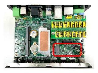
Step 2. Insert the M.2 Key B module at a 45-degree angle and insert it to the slot until the gold-pated connector of module contacted firmly with the slot.
