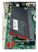
Step 3. Press the modules down until it's fixed firmly by the two locking latches on each side.
