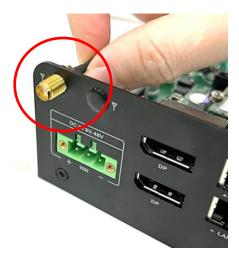
Step 3. Put on the washer and fasten the nut with the antenna jack.
