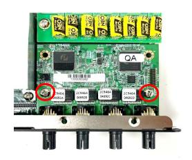
Step 5. Attach the assembled M12 I/O bracket on to the system, and fasten the hex nuts to fix it.
