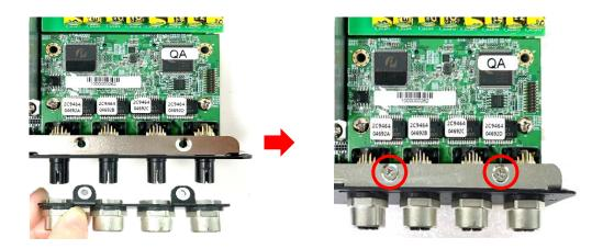
Step 6. Tie the rubber rings back to each M12 LAN port.
