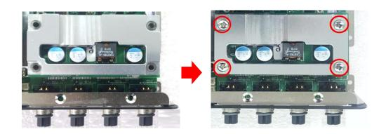
Step 7. Paste the last thermal pad onto the heatsink carefully, and then continue the step 5~ step 6 in chapter 3.14.3.
