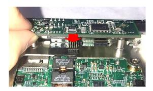
Step 3. Fasten the two screws to secure the power ignition board.
