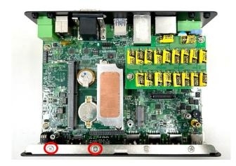
Step 3: Align the pins on the module with the connector on the right side as indicated, and then insert the CMI module vertically until it is securely connected with ensuring that the screw holes are properly aligned.
