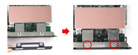
Step 8. Fasten the 4 D-Sub jack screws to fix the module. Then the installation of the module is complete.
