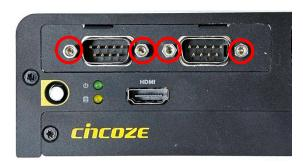
After installing CMI-COM05 module, users are required to navigate to BIOS > Advanced Setup > <u>F81966 Super IO Configuration</u> to verify the presence of the items related to the CMI-COM05 module, specifically 'Serial Port 3 Configuration' and 'Serial Port 4 Configuration'.
