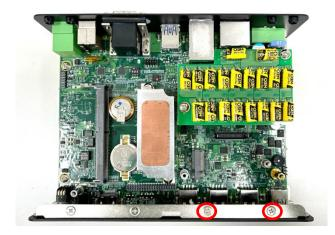
Step 3. Locate the chip place on the CMI-10GLAN module marked by red square. Paste the thermal pad on it carefully.
