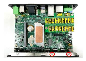
Step 3. Remove the four hex rings from the CMI-M12LAN module.
