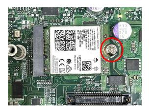
Step 4. Insert the CAP board with precision, ensuring that each pin is aligned with its corresponding hole on the socket. Secure the board in place by tightening the two screws.
