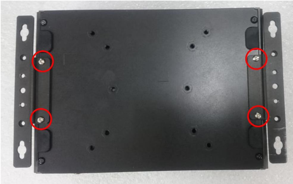
2. There are 2 bracket mounting holes at left and right side for customer fix the system on the wall.
