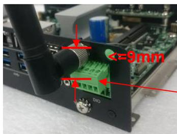
Terminal block connector on DIO ports
