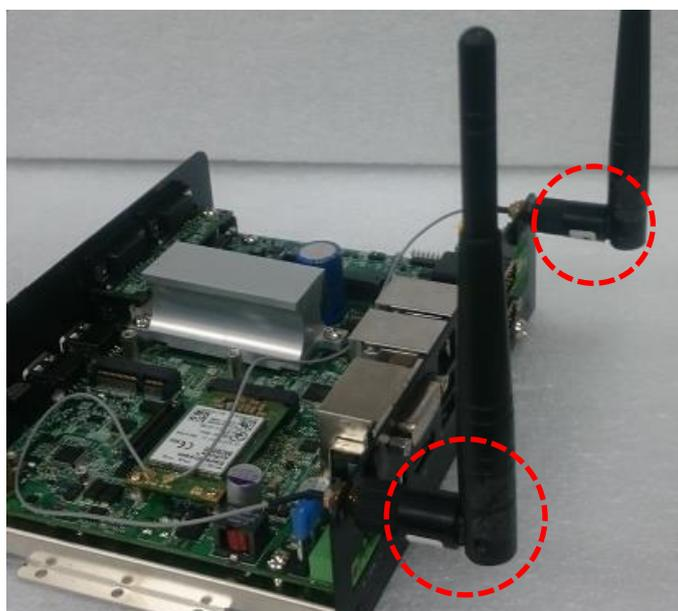
5. Attach the RF connector at another end of cable onto the module.
