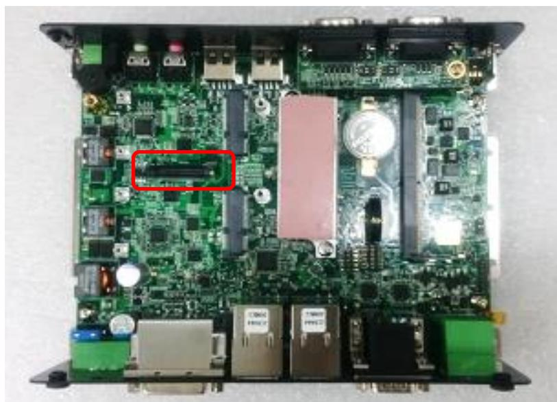
4. Insert the CMI module vertically into the female connector on system's mainboard until it's connected firmly. Fasten the 2 screws to fix it.
