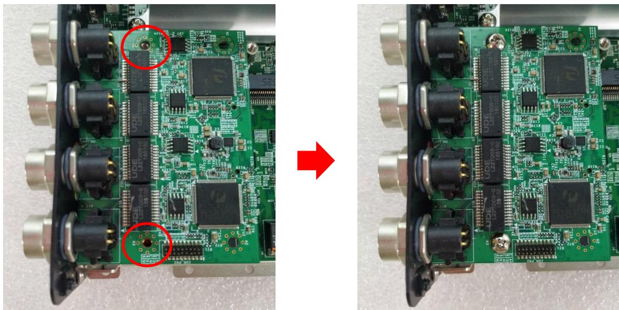
5. Fasten 2 screws on the front bezel.
