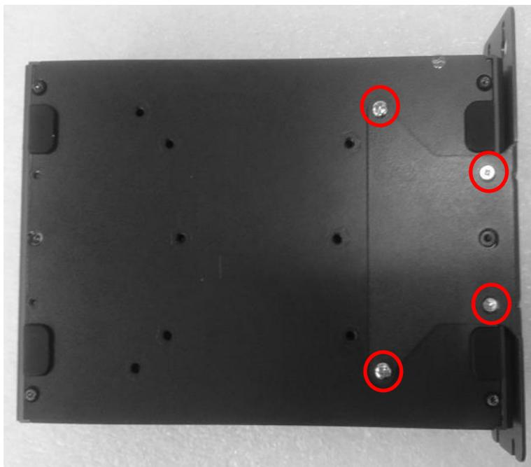
2. Fasten the screws through the bracket mounting hole to mount system on the wall.
