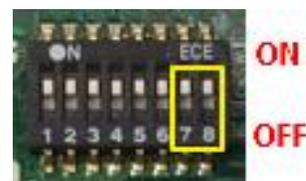
**MODE\_SEL6 / MODE\_SEL7 Pin Defined: COM6 / COM5 Power Select**
