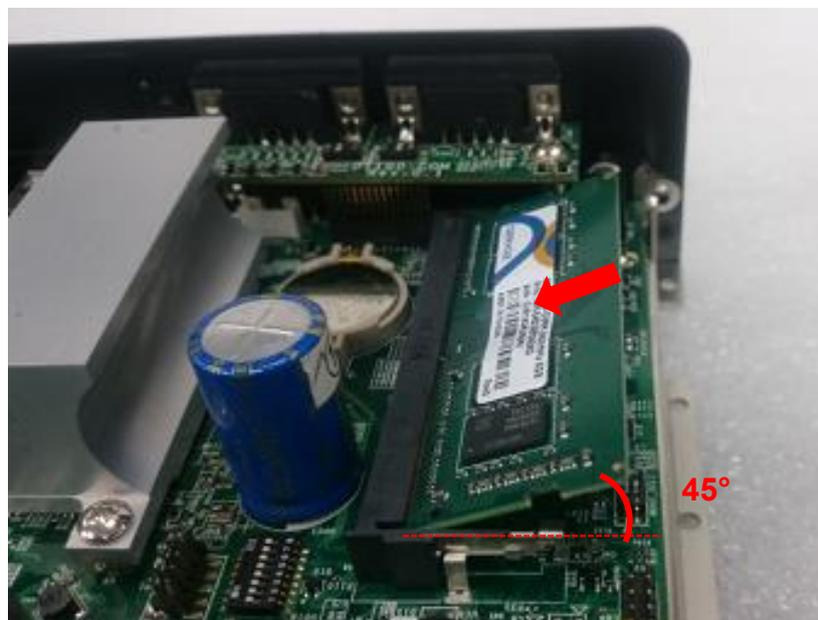
3. Press the modules down until it's fixed firmly by the two locking latches on the sides.
