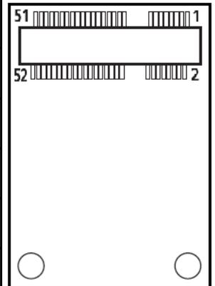
**MINIPCIE2: Mini PCI-Express Socket (Support mSATA and SIM Card to Link feature)**
