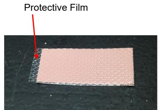
3. Paste the thermal pad onto the heatsink carefully.
