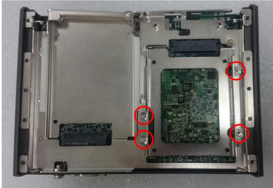
2. Make the bottom side of HDD face up, and place the HDD bracket on it. Ensure the direction of bracket is correct and use 4 provided screws to assemble HDD and HDD bracket together.
