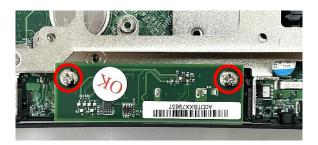
Step 4. Attach the I/O bracket on to the system, and fasten the screws to fix it.
