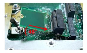
Step 4. Press down the module and fasten the screw to secure the module.
