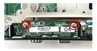
Step 4. Attach the I/O bracket and fasten the screws to fix it.
