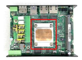
Step 2. Remove the protective film from one side of the Thermal Pad and then place the thermal pad onto the CPU heatsink.
