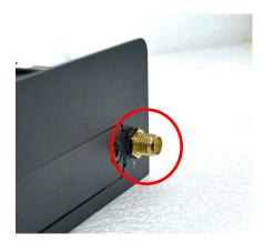
Step 4. Assemble the antenna and antenna jack together.
