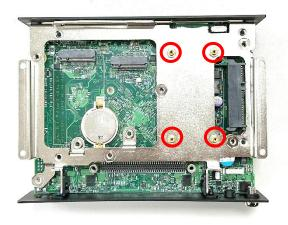
Step 3. Connect the Half Slim SSD to the SATA connector of the unit and fasten the 4 screws (M1.6x3, attached in the Screw Pack).
