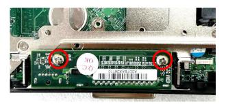
Step 5. Attach the I/O bracket on to the system, and fasten the screws to fix it.
