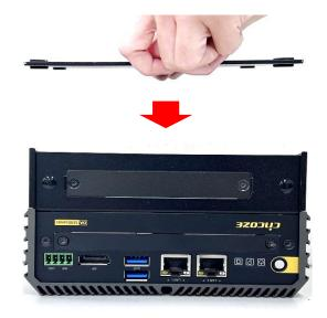
Step 7. Fasten the 4 screws back onto the bottom cover.
