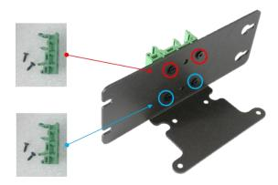
Step 2. Refer to Chapter 3.14 to install the side mounting bracket at a side of system.
