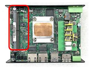
Step 2. Tilt the SO-DIMM module at a 45-degree angle and insert it to SO-DIMM socket until the gold-pated connector of module contacted firmly with the socket.
