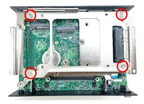
Step 2. Fasten the 4 copper pillars (M3X3, attached in the Screw Pack).
