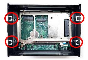
Step 5. Align the four hex standoffs with the holes on the expansion box, insert them through, and fasten them into the mounting holes on the system unit using a flathead screwdriver.
