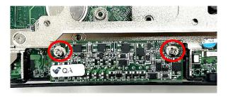
Step 4. Attach the I/O bracket and fasten the screws to fix it.
