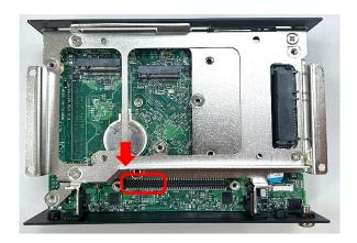
Step 3. Insert the CMI module vertically with aligning the pin holes. And then secure it with the two screws.
