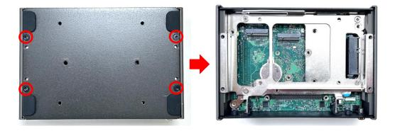
Step 2. Carefully place the expansion box onto the system unit according to the direction as shown below.
