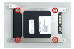
Step 3: Flip the HDD bracket over and connect it to the SATA connector, then fasten the four screws.
