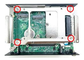
Step 2. Locate the M.2 Key B 3052 slot (socket CN1).
