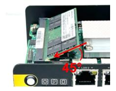
Step 3. Press the modules down until it's fixed firmly by the two locking latches on each side.
