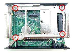
Step 2. Locate the M.2 Key B 3052 slot (CN1).
