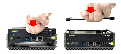
Step 2. Fasten the 4 screws back to the bottom panel of the system.
