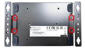
Step 2. The indicated two mounting holes at left and right sides are designed to fix the system on the wall.
