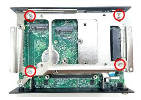
Step 2. Make the PCB side of the HDD face up, place the HDD bracket on it. Ensure the direction of bracket is correct and use 4 provided screws to assemble HDD and HDD bracket together.
