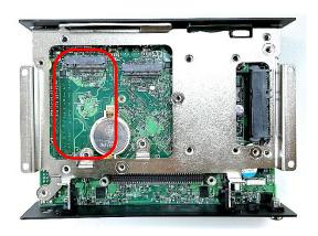
Step 3. Place the M.2 Key B Type 3052 to 3042 Adapter Bracket with aligning the corresponding screw hole, and then fasten the screw.
