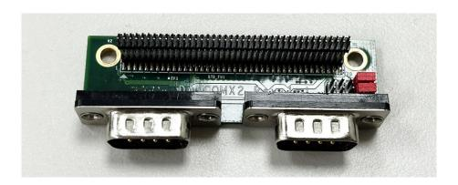
COM3 and COM4 (on the module): COM Port Connector (Support RS232/RS422/RS485)
