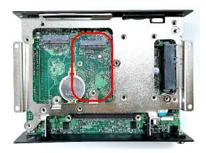
Step 3. Insert the M.2 Key B module at a 45-degree angle and insert it to the slot until the gold-pated connector of module contacted firmly with the slot.
