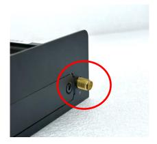
Step 3. Put on the washer and fasten the nut with the antenna jack.
