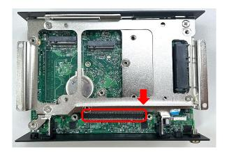
Step 3. Thread the module through the cavity designated for I/O bracket with an inclined angle and insert the CMI module vertically with aligning the right 76 pin holes.
