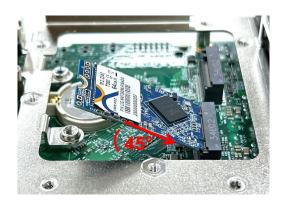
Step 4. Press down the module and fasten the screw to secure the module.
