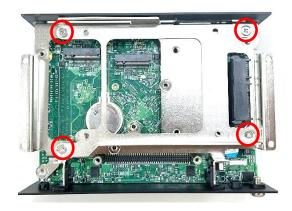
Step 2. Fasten the 4 copper pillars (M3X3, attached in the Screw Pack).
