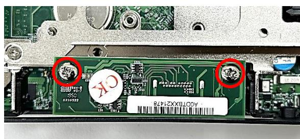
Step 4. Attach the I/O bracket on to the system, and fasten the screws to fix it.
