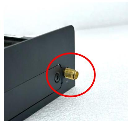
Step 3. Put on the washer and fasten the nut with the antenna jack.
