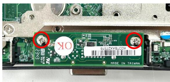
Step 4. Attach the I/O bracket on to the system, and fasten the screws to fix it.
