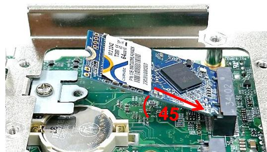
Step 5. Press down the module and fasten the screw to secure the module.
