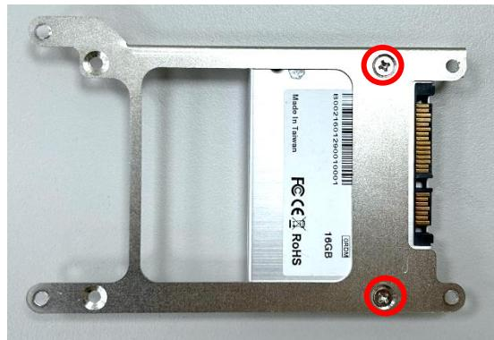
Step 3: Flip the HDD bracket over and connect it to the SATA connector, then fasten the four screws.
