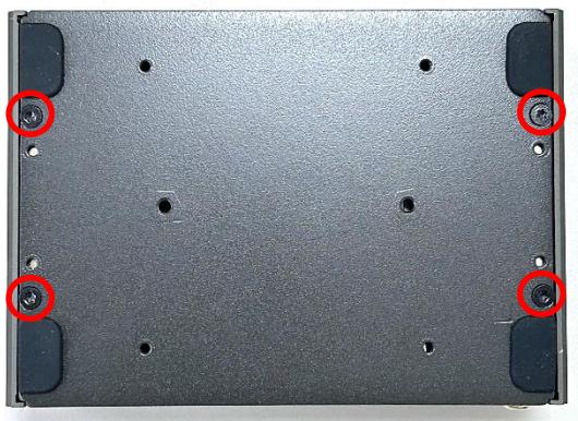
Step 2. Remove the bottom panel and then the system body from the chassis.
