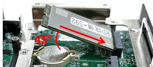
Step 4. Press down the module and fasten the screw to secure the module.
