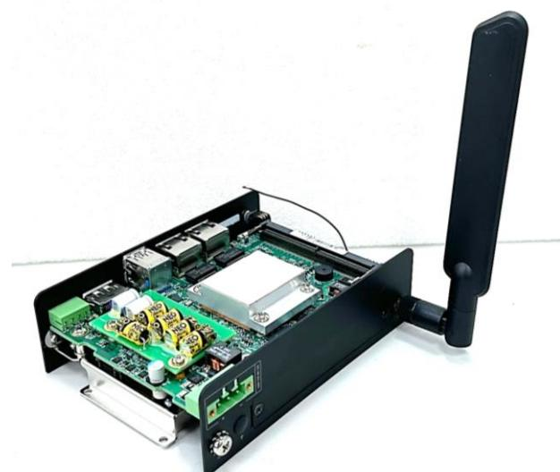
Step 5. Attach the RF connector at another end of cable onto the module.
