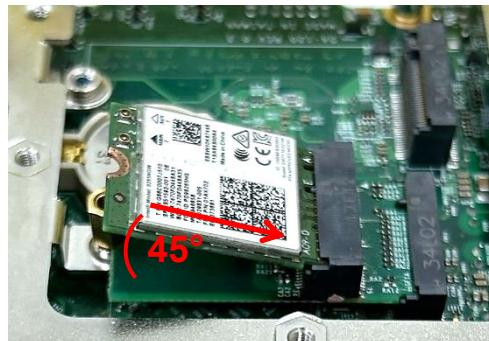
Step 6. Press down the module and fasten the screw to secure the module.
