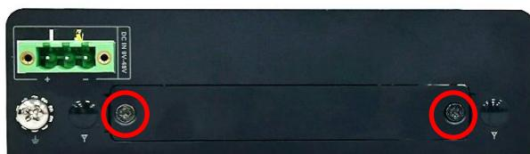
Step 2. Attach the I/O bracket on to the system, and fasten the screws to fix it. For guidance on antenna installation methods, please refer to Chapter 3.4.
