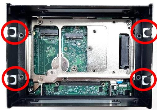
Step 5. Align the four hex standoffs with the holes on the expansion box, insert them through, and fasten them into the mounting holes on the system unit using a flathead screwdriver.
