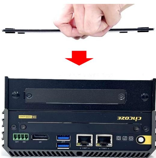
Step 7. Fasten the 4 screws back onto the bottom cover.
