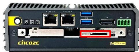
Step 3. Insert the SIM card into the SIM slot(s) with the gold contacts facing up. Please pay attention to the insert orientation as illustrated.
