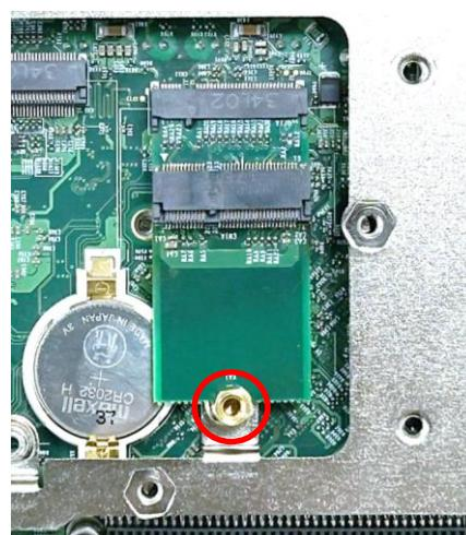
Step 5. Insert the M.2 Key E module at a 45-degree angle and insert it to the slot until the gold-pated connector of module contacted firmly with the slot.
