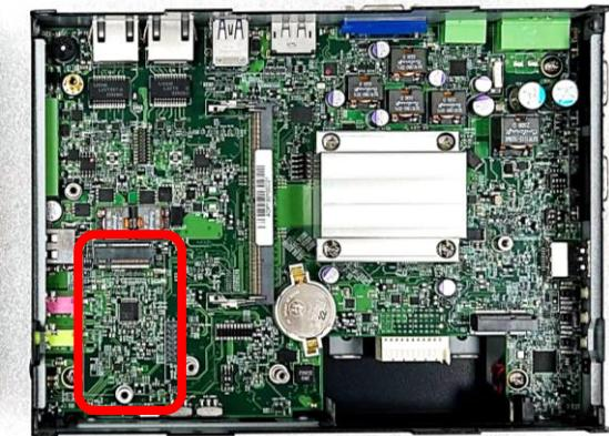
Step 2: Align the M.2 Key B Type 3052 to 3042 Adapter Bracket with the corresponding screw hole. Secure the bracket in place and fasten the screw.
