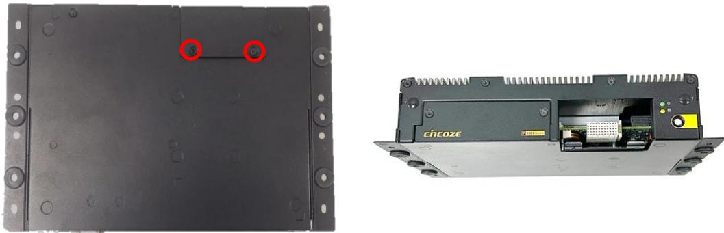
Step 3. Locate the male connector (on the display module) and the female connector (on the system).
