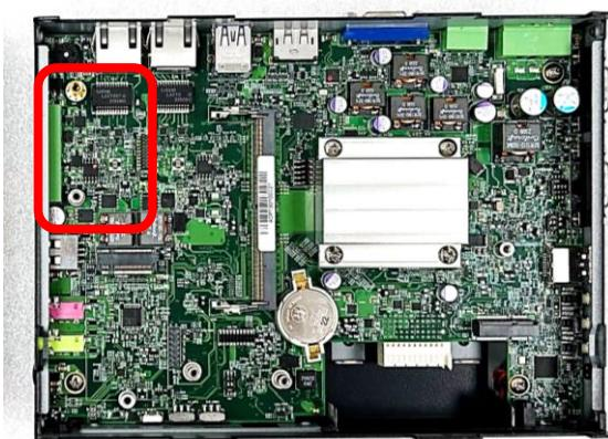
Step 2. Insert the female connector of CFM-PoE module to the male connector on system motherboard.
