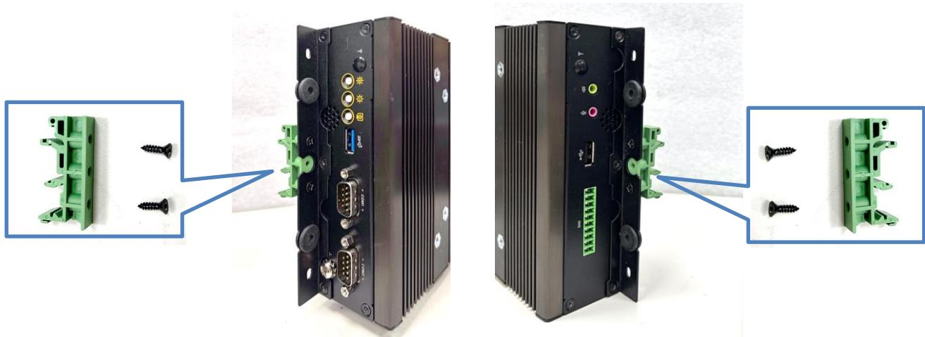
Step 3. Clip the system into DIN rail as illustrated by the following steps. (1) Have upper end of mounting clip snaps into the DIN rail. (2) Press the system toward to have lower end of mounting clip snaps into the other side of DIN rail.
