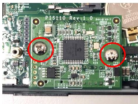
Step 3. Loosen the 2 screws on front panel to remove cover plate.
