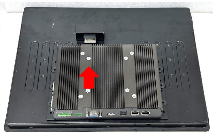
Step 5. Fasten the 6 screws to fix the system on the display module.
