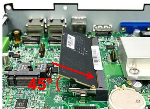
Step 3. Press the modules down until it's fixed firmly by the two locking latches on each side.
