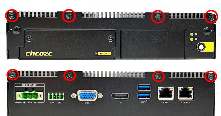
Step 2. Remove the cover from the chassis.
