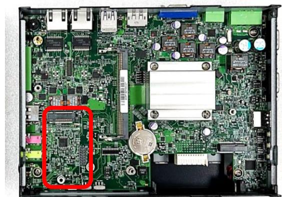
Step 2. Insert the M.2 Key B card at a 45-degree angle and insert it to the slot until the gold-pated connector of module contacted firmly with the slot.
