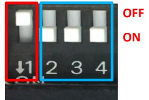
Default setting of Pin1 to Pin4 is OFF/ON/ON/ON.
