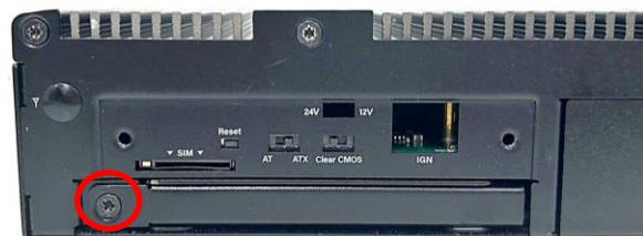
Step 7. Fasten the 2 screws on the front panel.
