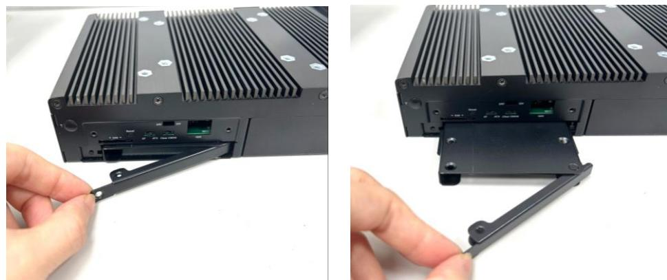
Step 4. Make the bottom side of the HDD face up, place the HDD bracket on it. Ensure the direction of bracket is correct and use 4 provided screws to assemble HDD and HDD bracket together.
