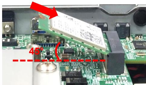
Step 3. Press the card down and secure it with one screw.
