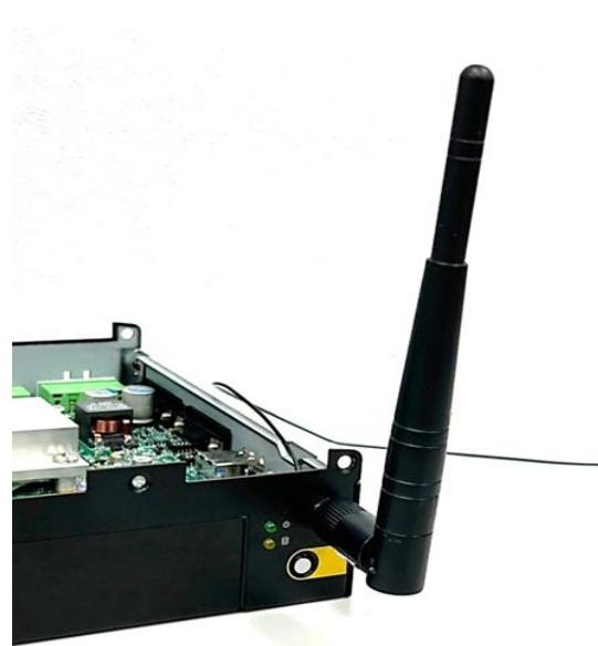
Step 5. Attach the RF connector at another end of cable onto the module.
