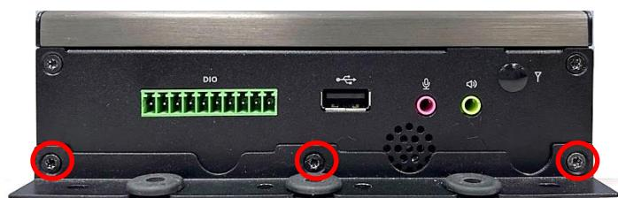
Step 4. Attach the system to the wall by fastening four screws through the mounting holes at each side as illustrated.
