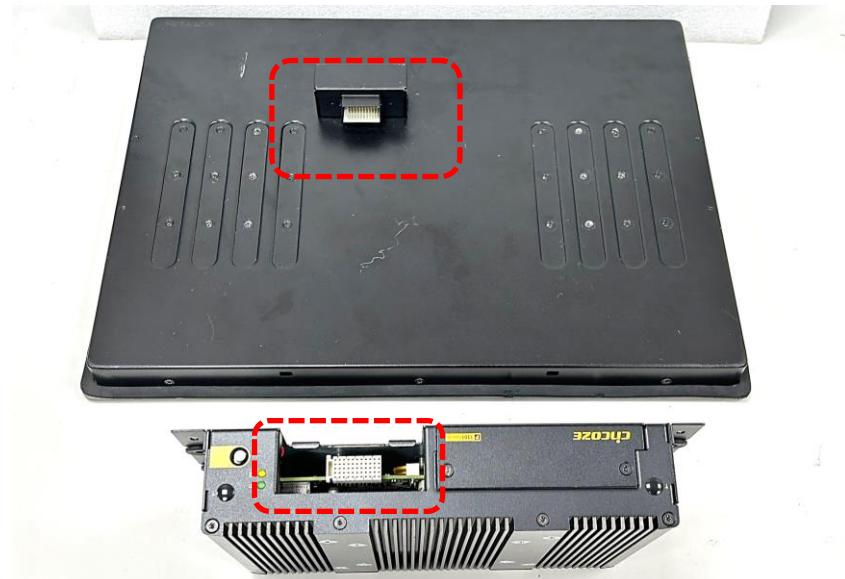
Step 4. Align the two connectors to connect them together as illustrated below.
