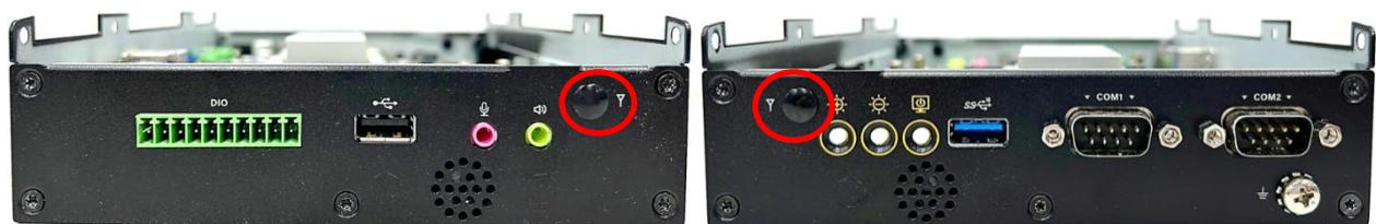
Step 2. Have the antenna jack penetrate through the hole.
