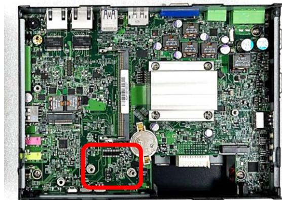
Step 2. Insert CFM-IGN module vertically to the female connector on the system's mainboard, and fasten the 2 screws to fix it.
