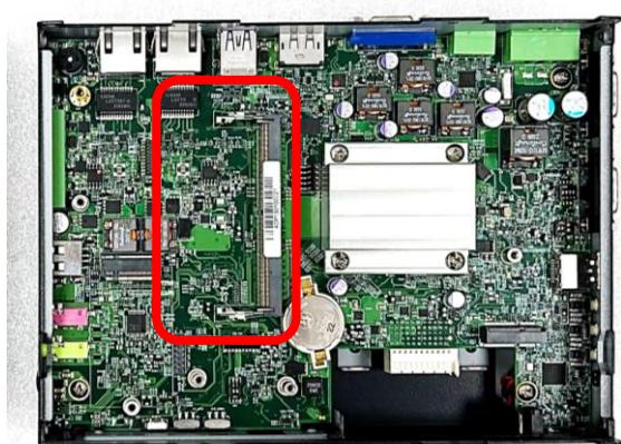
Step 2. Tilt the SO-DIMM module at a 45-degree angle and insert it to SO-DIMM socket until the gold-pated connector of module contacted firmly with the socket.
