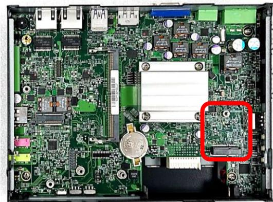
Step 2. Tilt the M.2 Key E card at a 45-degree angle and insert it to the socket until the golden finger connector of the card seated firmly.
