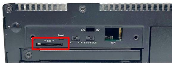
Step 3. Insert the SIM card until you hear a click sound; that indicates the installation is complete.
