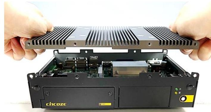
Step2. Fasten the 8 screws to fix the cover.
