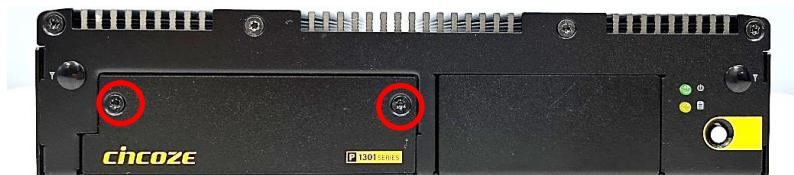
Step 2. Loosen the screw on the HDD bracket.
