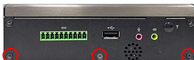
Step 3. Assemble two wall mount brackets by fastening three screws on each side.
