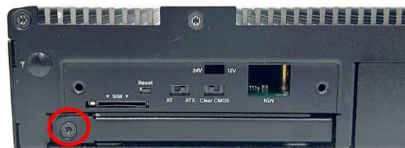
Step 3. Pull out the HDD bracket.
