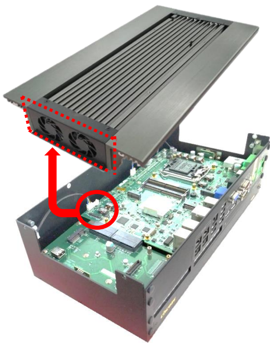
POWER1 (FAN OUT Control)
