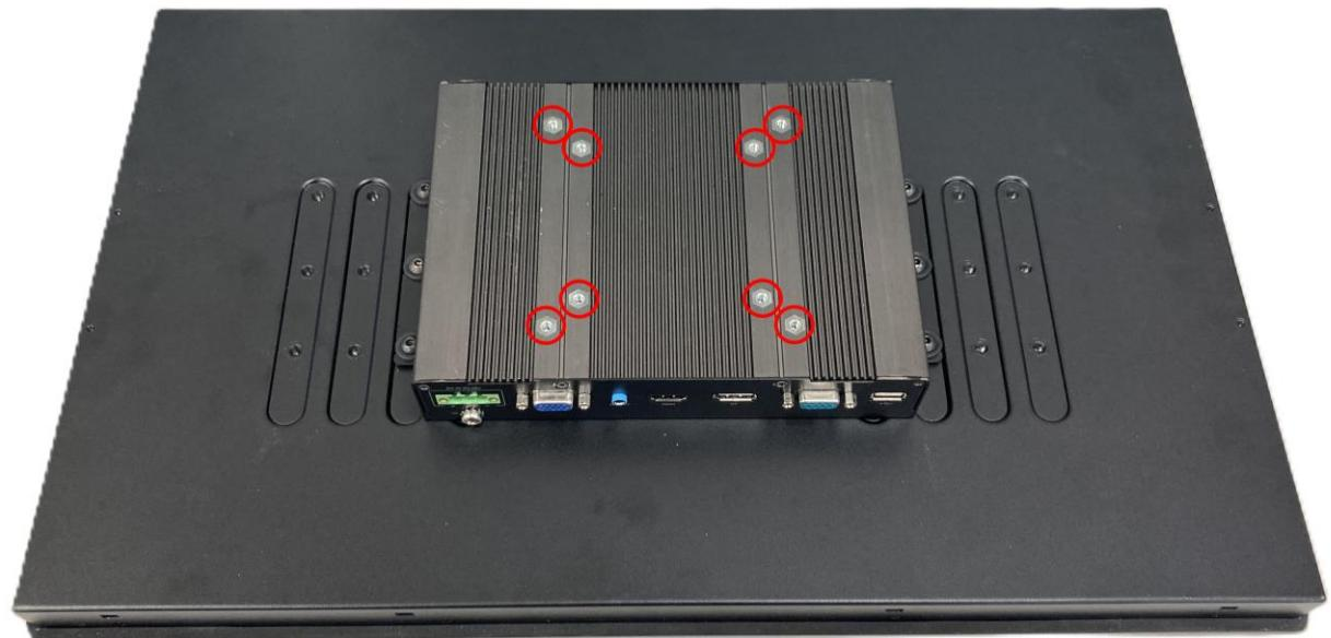
Step 1. Place the VESA stand on top of the monitor module and align the holes on the stand with the holes on the top side of M1101.
