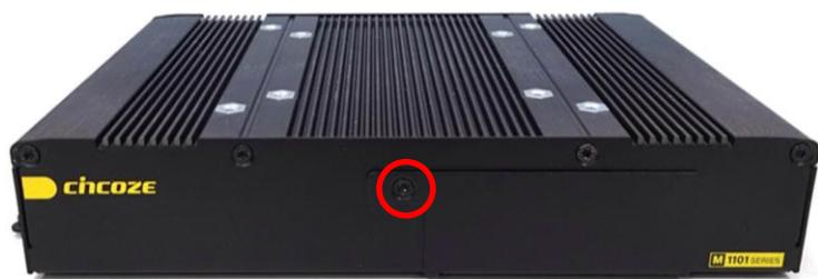
Step 2. Turn over the module and loosen 2 screws at the back of the connector cover.
