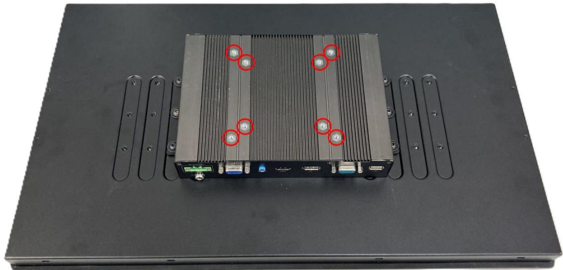
Step 1. Align the rack mount base with the VESA screw holes as shown below and secure it with screws.
