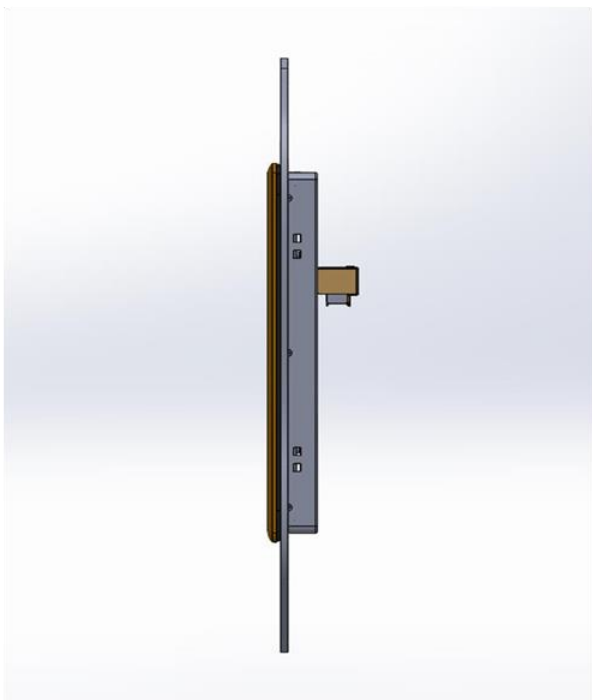
Panel mount side view with LVDS connector
