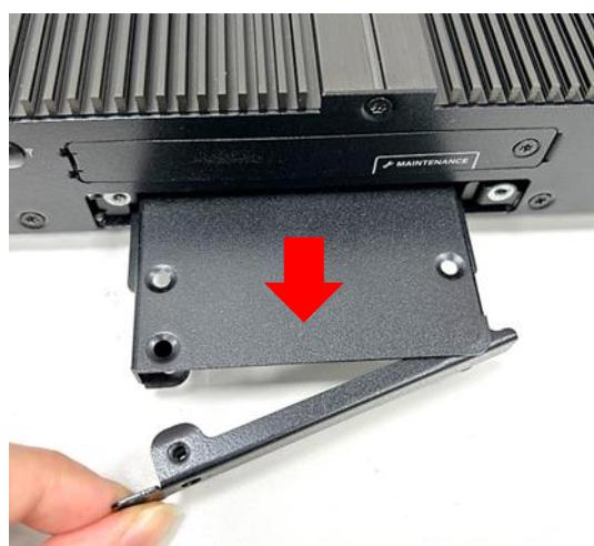
Step 5. Place the HDD bracket on screw-hole side of HDD. Use four screws provided to assemble HDD on the bracket.
