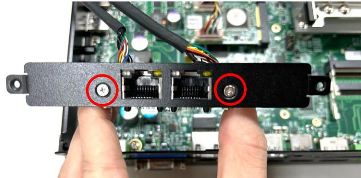
Step 9. Attach the MEC-LAN bracket, and fasten the 2 screws to fix it as indicated.
