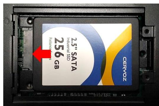
Step 6. Secure the HDD bracket with three screws.
