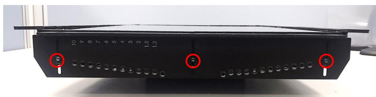
Step 8. Locate the top and bottom-side mounting brackets.
