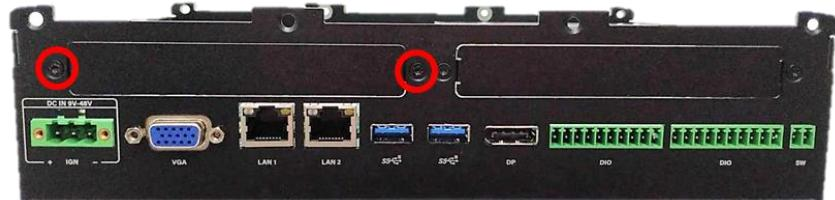
Step 2. Attach the PCI / PCIe Card Installation Kit on, and fasten the two screws back on rear panel to fix the Kit.
