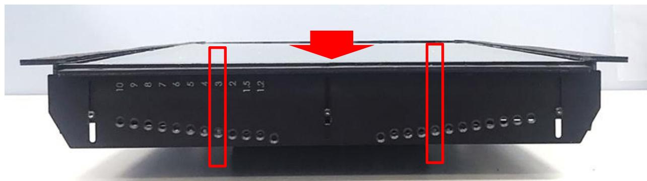
Step 6. Fasten the two screws on the left and right-side mounting brackets.
