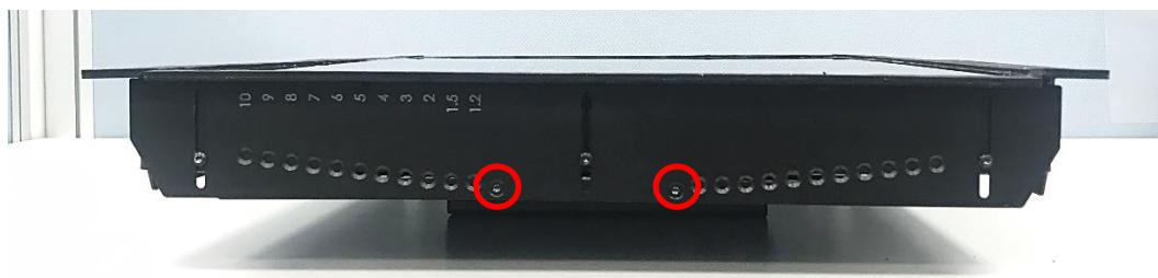
Step 3. Loosen the three screws on the left and right-side mounting brackets.
