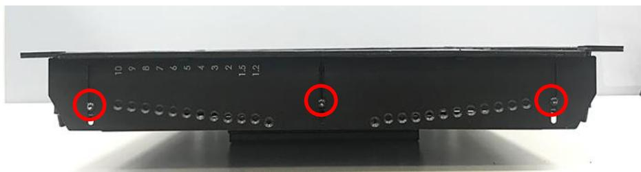
Step 3. Remove the 3 screws on the top and bottom side of mounting brackets.
