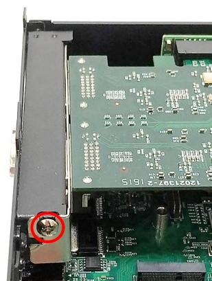
Step 7. Loosen the two screws as indicated to have the clamp arm slideable.
