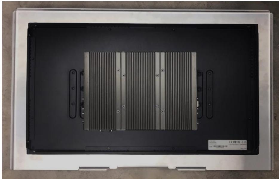
There are two methods for fastening the CO-100/P2202 module onto the cabinet to complete the flat mount. One is to fix the CO-100/P2202 module from the front side of the cabinet, which is illustrated in chapter 3.16.1. The other one is to fix the CO-100/P2202 module from the rear side of the cabinet, which is illustrated in chapter 3.16.2.
