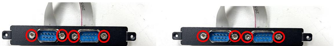
Step 8. Attach the MEC-COM bracket, and fasten the 4 screws to fix it as indicated.
