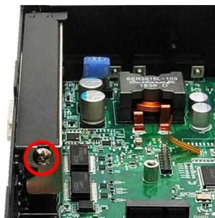
Step 4. Align the notch of golden fingers of Riser card (Optional) with the slot. Insert the card vertically, and press the card straight down into the slot until it's seated firmly.
