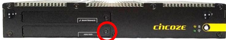
Step 2. Loosen the screw as indicated on the HDD bracket.
