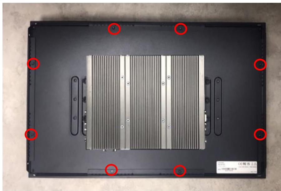
Step 2. Remove the 3 screws on the left and right side of mounting brackets.
