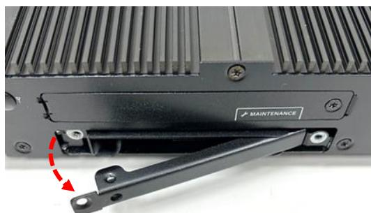
Step 4. Hold the rotating arm to pull out the HDD bracket.
