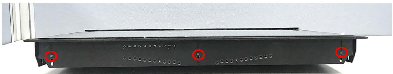
Step 14. Put the CO-100/P2202 module onto the rack back side.
