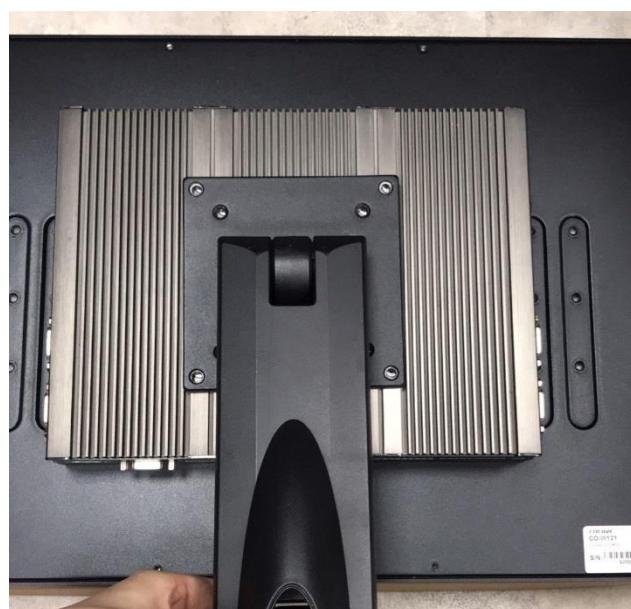
Step 2. Fasten the VESA mount screws to complete the VESA mounting.
