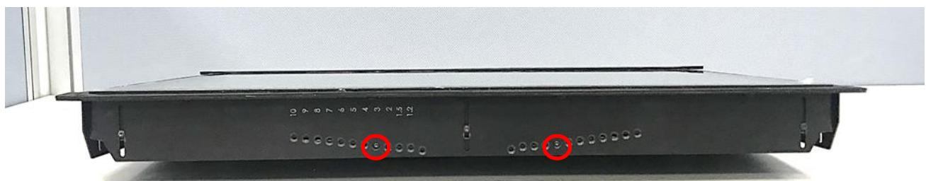
Step 13. Fasten the three screws on the top and bottom-side mounting brackets.
