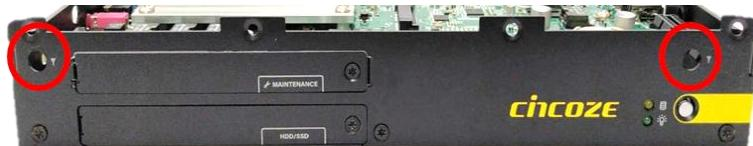
Step 2. Penetrate the antenna jack through the hole. And then put on the washer and fasten the nut with antenna jack.
