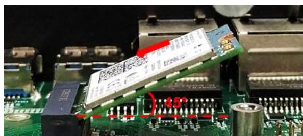
Step 3. Press the card down and secure it with 1 screw.
