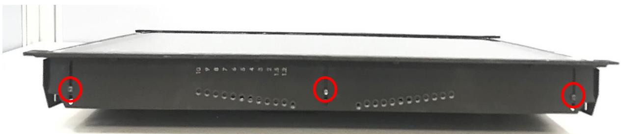
Step 4. Remove the four mounting brackets.
