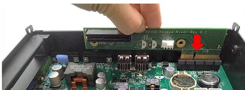
Step 5. Align the notch of golden fingers of PCI(e) card with the expansion slot. Insert the card horizontally, and press the card straight down into the slot until it's seated firmly.
