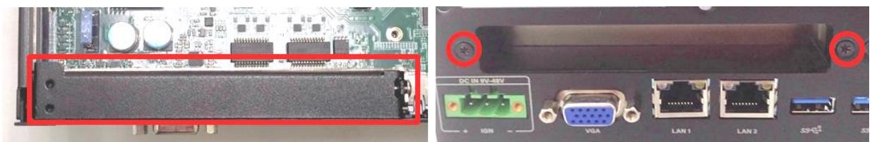
Step 3. Loosen the screw as indicated to remove the PCI bracket.
