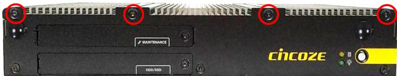
Step 2. Raise the top cover and remove it from the chassis.
