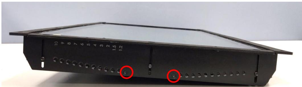
Step 1. Put the CO-100/P2202 module onto the rack's back side.
