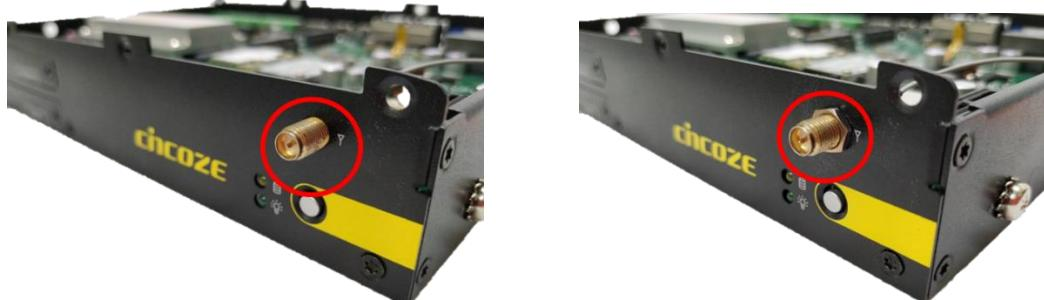
Step 3. Assemble the antenna and antenna jack together.
