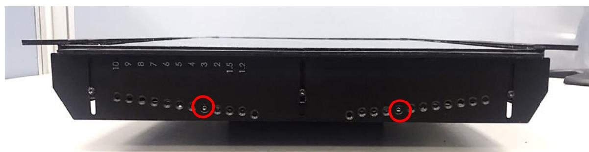
Step 7. Fasten the three screws on the left and right-side mounting brackets.
