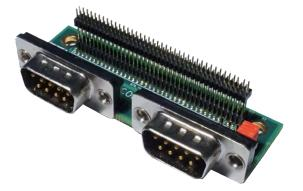
CMI Module with 2x RS232/422/485 Ports (Support 5V/12V), 2x DB9 Connector
