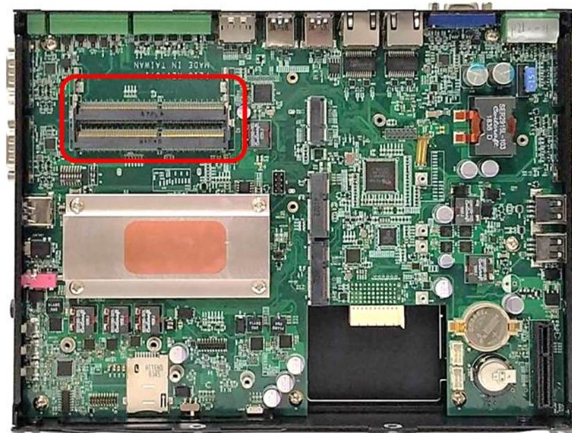
2. Tilt the memory module at a 45-degree angle, and insert it into SO-DIMM socket until the golden finger connector of the module is seated firmly.
