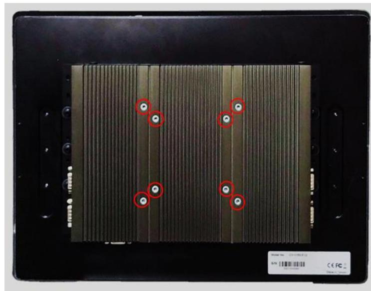
1. The following picture uses a panel PC (P2102+CV/CS display module) as a demonstration. To attach the panel PC to a VESA stand, please fasten eight screws as indicated to fix it on the stand.
