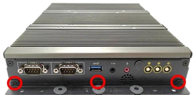
4. Turn over the system to bottom side. Locate the connector cover of display module.
