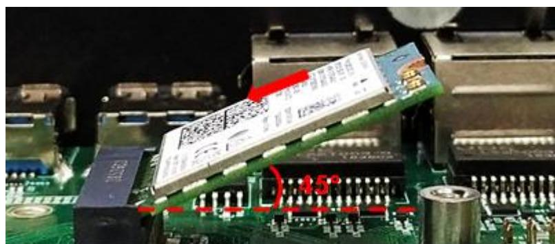
3. Press the card down and secure it with 1 screw.
