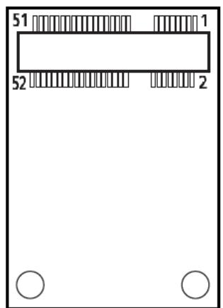
**CN3 : M.2 Key E Socket (Support M.2 PCIE / Intel CNVi )**
