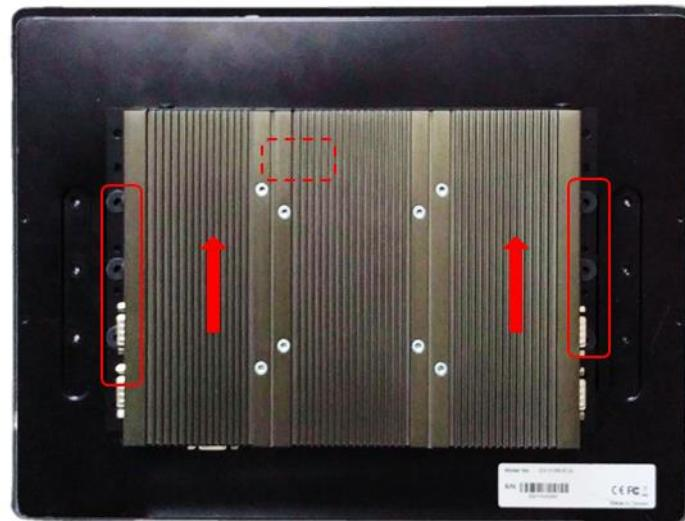
8. Fasten six screws to secure P2102 on the display module.
