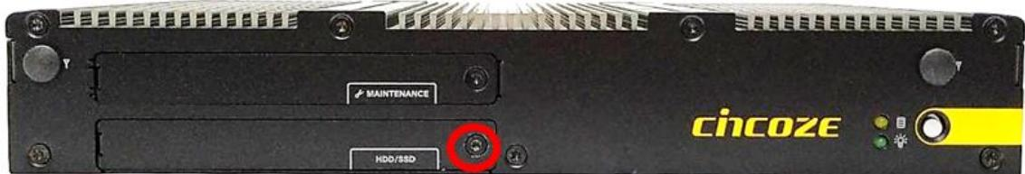
8. Fasten the screw to secure the HDD bracket on the system chassis.
