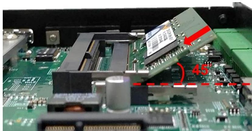
3. Press down the memory module until retaining clips snap back in place.
