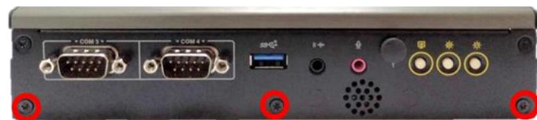
3. Assemble two mounting brackets by fastening six screws from the screws pack.
