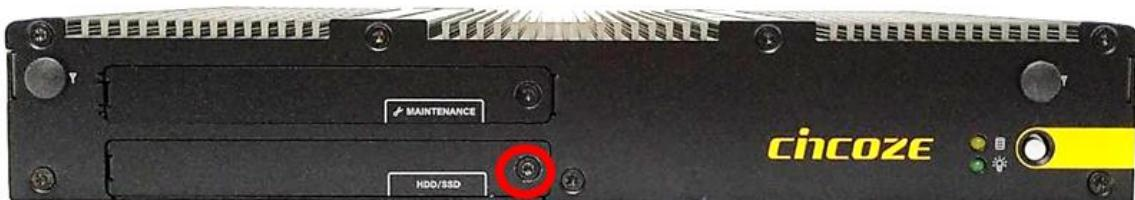
3. Pull the rotating arm of HDD bracket outward as indicated.
