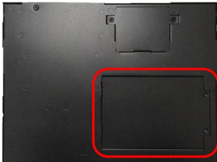
2. Loosen the two screws, lift the cover, and then remove it.
