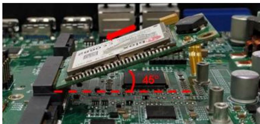
3. Press the card down and secure it with 2 screws.
