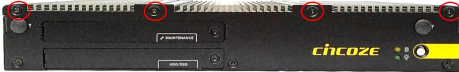
2. Raise the edge of top cover (1), and raise the other side (2) subsequently to remove it from the chassis.
