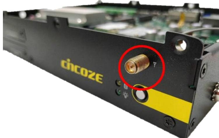
3. Put on the washer and fasten the nut with antenna jack.
