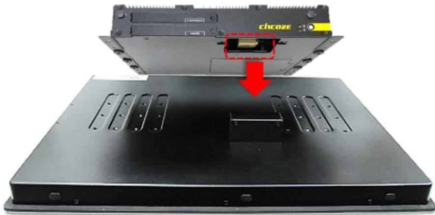
7. Align the mounting holes of P2102 with the screw holes of display module underneath. Then slide the PC2100 carefully as indicated to have P2102 and display module connected together.
