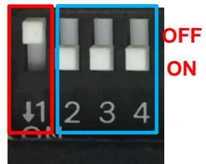
Default setting of Pin1 to Pin4 is OFF/ON/ON/ON.
