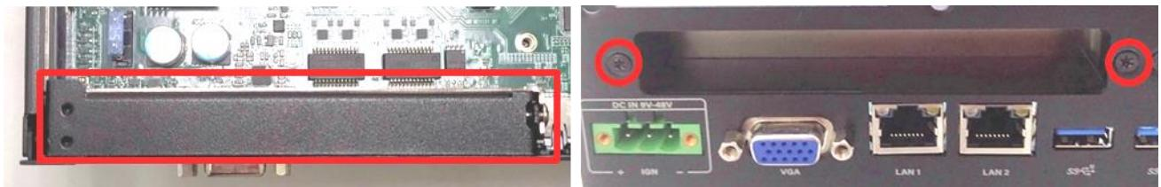
3. Loosen the screw as indicated to remove the PCI bracket.
