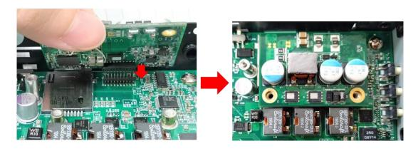
6. Put on the PoE thermal block and fasten two screws to secure the PoE board.
