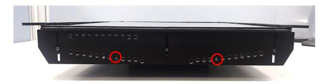
7. Fasten the three screws on the left and right-side mounting brackets.
