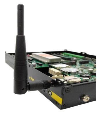
5. Attach the RF connector at another end of the cable onto the card.
