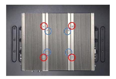
1. Put the VESA stand on, and align with the mounting holes.
