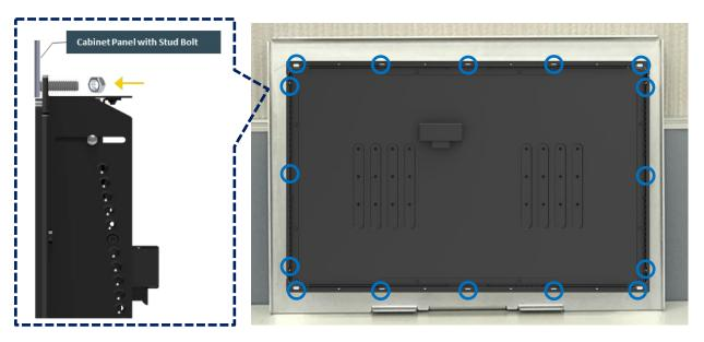
If the cabinet panel is with bosses as the following figures, user can prepare 16 pcs of M4 screws for fixing the module through the **oblong holes** (oblong hole size: 9mmx 4mm, without screw thread).
