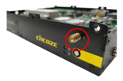
3. Put on the washer and fasten the nut with antenna jack.
