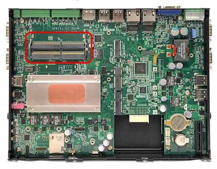
2. Tilt the memory module at a 45-degree angle, and insert it into SO-DIMM socket until the golden finger connector of the module is seated firmly.
