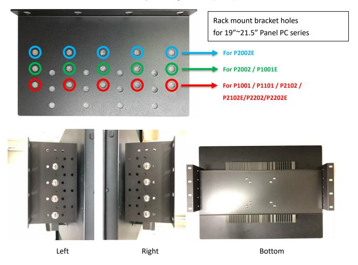
4. Assemble two rack mount brackets by fastening 4 screws (M5x12), flat washers and hex nuts at each side.
