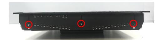
3. Remove the 3 screws on the top and bottom side of mounting brackets.
