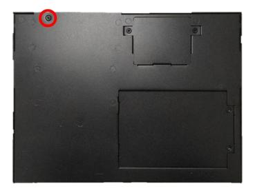
2. Loosen the screw to remove the HDD bay cover bracket.
