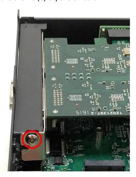
7. Locate the retention module of PCI(e) expansion card.
