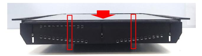
6. Fasten the two screws on the left and right-side mounting brackets.
