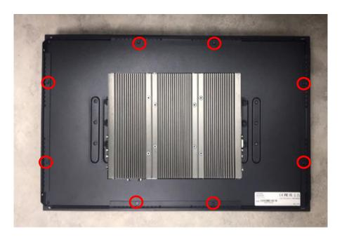
2. Remove the 3 screws on the left and right side of mounting brackets.
