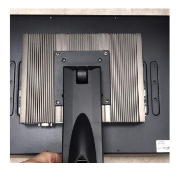
2. Fasten the VESA mount screws to complete the VESA mounting.
