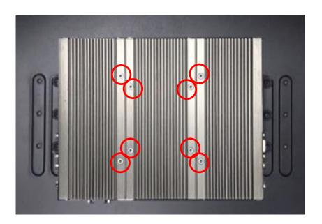
2. Put on the rack mount base and fasten the screws.
