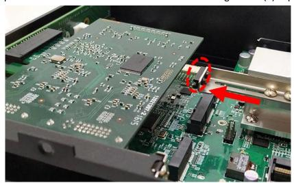
10. Finally, fasten the two screws that were previously loosen halfway to fix the retention module.
