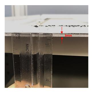
5. According to the thickness = 3mm for the example, push down the left and right-side mounting brackets to the place at screw hole = 3mm.
