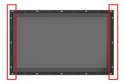
2. Remove the two screws on the left and right-side mounting brackets.
