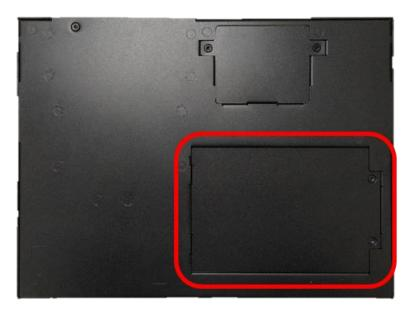
2. Loosen the two screws, lift the cover, and then remove it.
