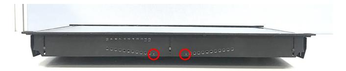
10. Loosen the three screws on the top and bottom-side mounting brackets.
