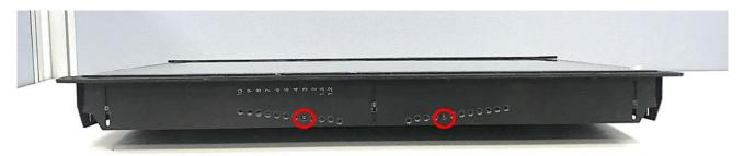
13. Fasten the three screws on the top and bottom-side mounting brackets.
