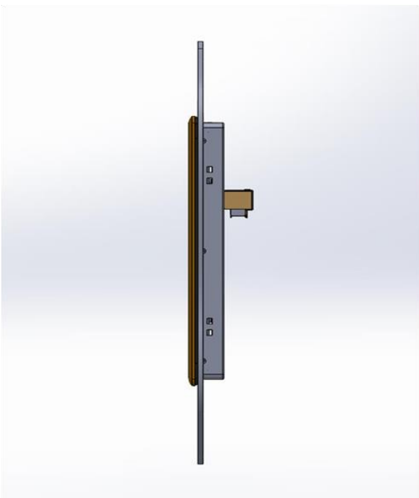
Panel mount side view with LVDS connector
