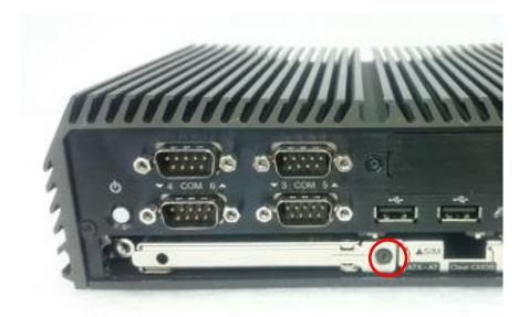
3. Pull the rotating arm and pull the HDD bracket out of system.
