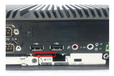
2. Insert a SIM card into SIM slot with the gold contacts facing up. Please pay attention to the insert orientation as illustrated.
