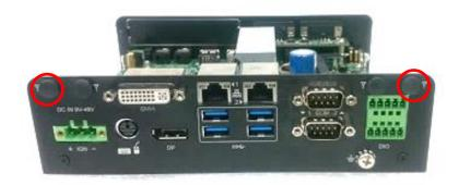
2. Penetrate the antenna jack through the hole at both sides as illustrated.
