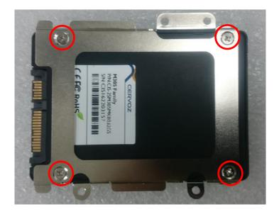
3. Turn over the HDD bracket assembly. Connect the HDD bracket to the SATA connector and fasten the 4 screws to fix it.
