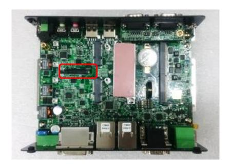
4. Insert the CMI module vertically into the female connector on system's mainboard until it's connected firmly. Fasten the 2 screws to fix it.
