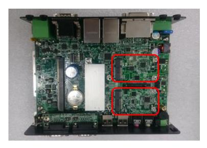
2. Insert the Mini-PCIe card at a 45-degree angle until its edge connector is connected firmly into slot.
