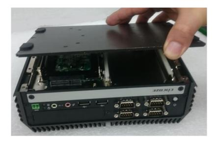
3. Hold front and rear panel and lift up the body of unit vertically.
