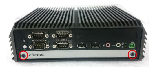
2. Locate the removable HDD bay and loosen the screw.
