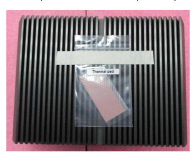
2. Remove the protective film on the thermal pad.
