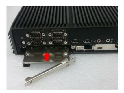
6. Place the rotating arm back and fasten the screw.
