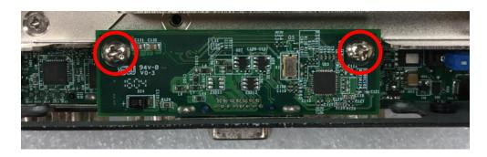
3. Attach the CMI-VGA bracket, fasten 2 screws and 2 D-Sub jack screws as marked on photo.
