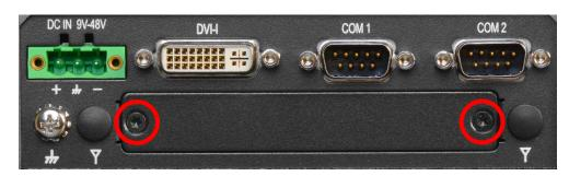
2. Insert CMI-VGA module vertically to the female connector on the system's mainboard, and fasten 2 screws to fix it.
