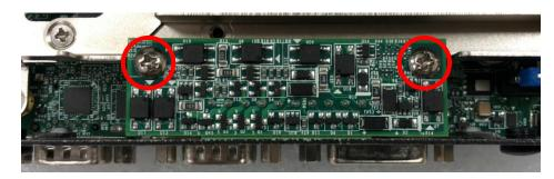
3. Attach the CMI-DIO bracket, and fasten 2 screws as marked on photo.
