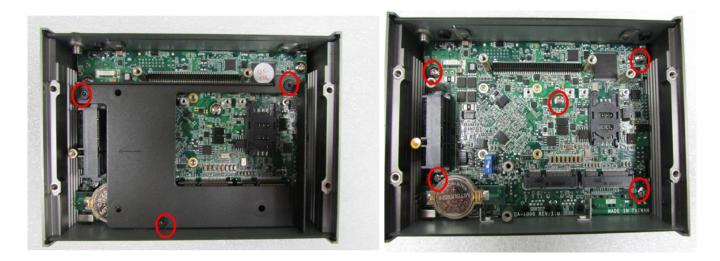
4. Hold front and rear panel and lift up the body of unit vertically.
