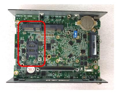
4. Tilt the Mini PCIe card at a 45-degree angle and insert it to the socket until the golden finger connector of the card seated firmly.
