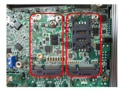
3. Insert the Mini-PCIe card at a 45-degree angle and insert it to the slot until the gold-pated connector of module contacted firmly with the slot.
