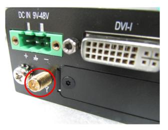
3. Put on washer and fasten the nut with antenna jack.
