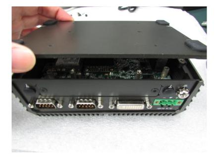
3. Loosen the 3 screws (left picture) and remove HDD base plate. Loosen the 5 screws (right picture) as marked on photo and place them aside.
