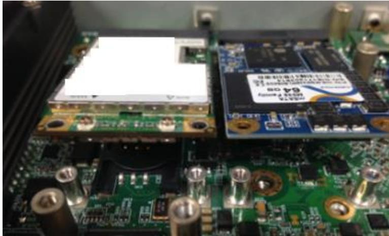
4. Press down the module and fasten two screws to secure the module.
