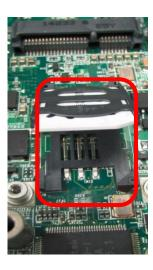
3. Press down the socket of SIM card to lock the location.
