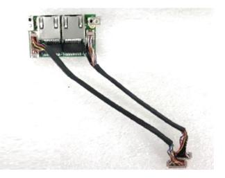
7. Attach the LAN board onto the back side of the cover plate, and then fasten the two screws to secure the module.
