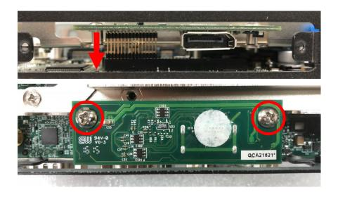
3. Attach the CMI-DP bracket, and fasten 2 screws as marked on photo.
