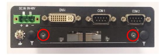
3. Remove the HDD bracket according to the step 1 in Chapter 3.4, and locate the Mini PCIe socket(s) on the bottom side of the system.
