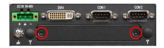
2. Insert CMI-DVI module vertically to the female connector on the system's mainboard, and fasten 2 screws to fix it.
