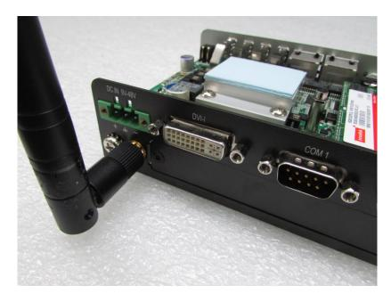
5. Attach the RF connector at another end of cable onto the module.
