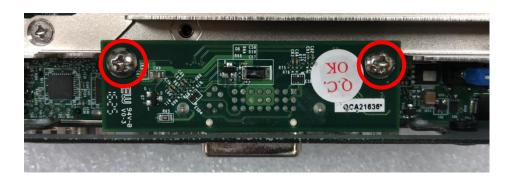
3. Attach the CMI-DVI bracket, and fasten 2 screws as marked on photo.
