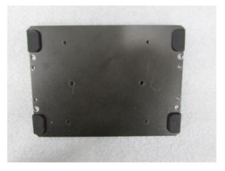
1. Provided below is the base of the system unit and screw holes specified to be mounted from VESA stand.
