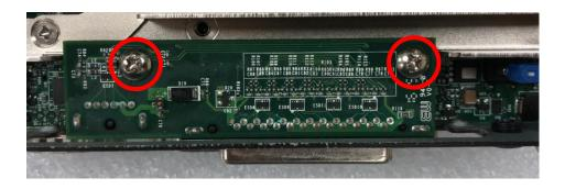
3. Attach the CMI-LPPS bracket, fasten 2 screws and 2 D-Sub jack screws as marked on photo.
