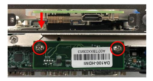
3. Attach the CMI-HD bracket, fasten 2 screws as marked on photo.
