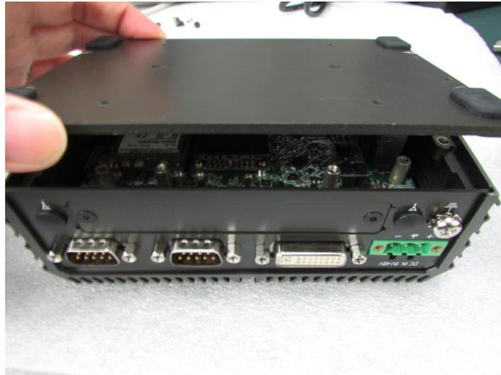
4. Fasten the 4 screws to fix the cover.
