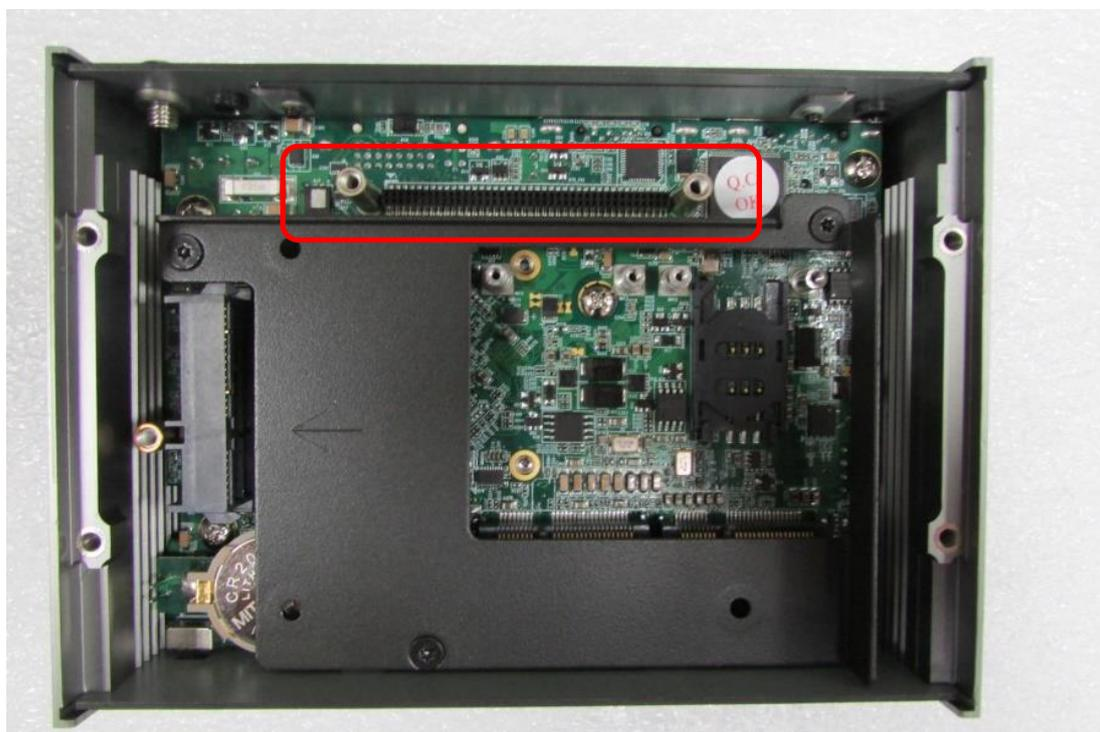
Locate the CMI connector on system motherboard as indicated.
