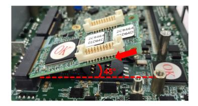
5. Press the card down and secure it with 2 screws.
