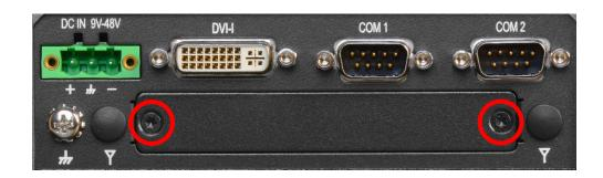
2. Insert CMI-DIO module vertically to the female connector on the system's mainboard, and fasten 2 screws to fix it.
