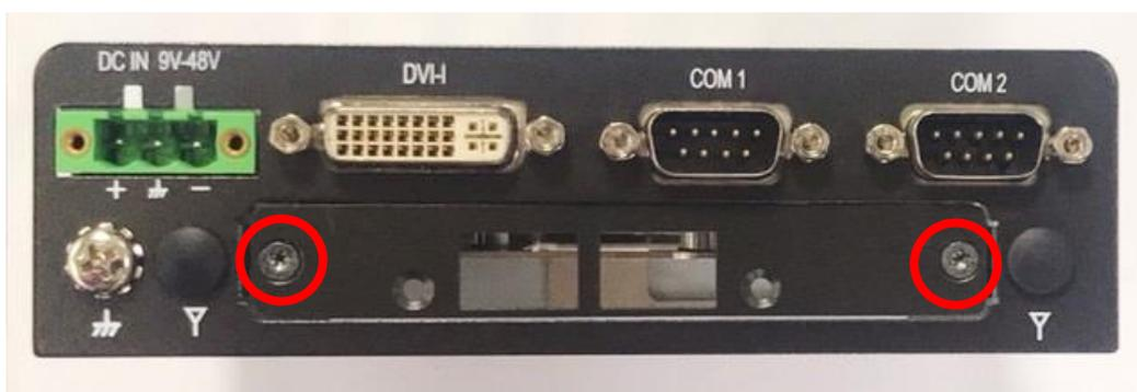
3. Remove the HDD bracket according to the step 1 in Chapter 3.4, and locate the Mini PCIe socket(s) on the bottom side of the system.
