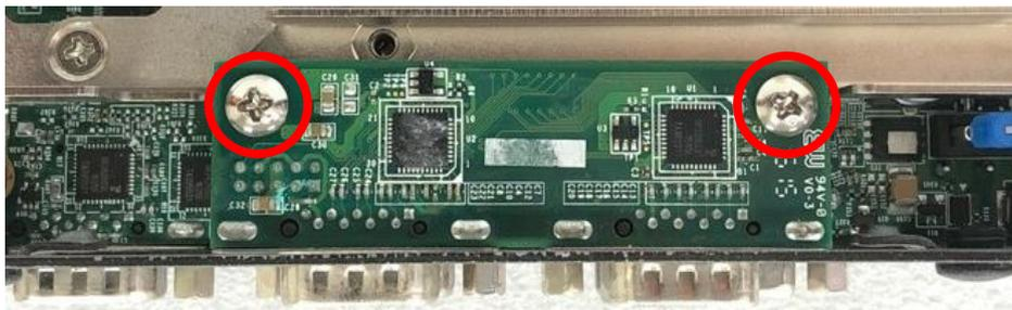
3. Attach the CMI-COM bracket, and fasten 2 screws as marked on photo.
