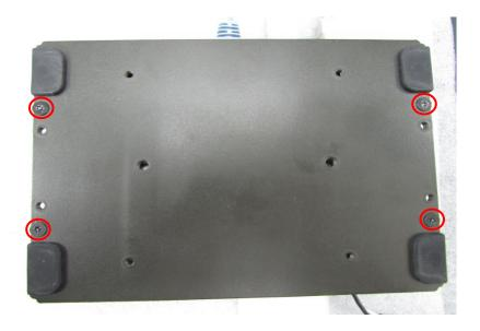
2. Remove the bottom cover from the chassis.
