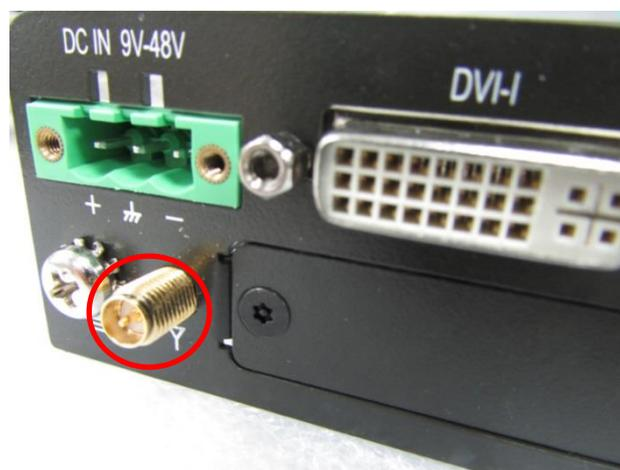
3. Put on washer and fasten the nut with antenna jack.
