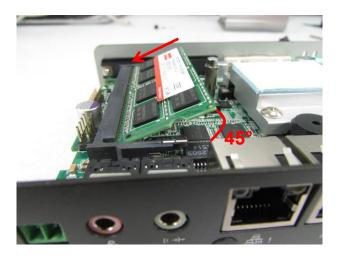
3. Press the modules down until it's fixed firmly by the two locking latches on the sides.
