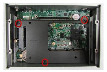
2. Put on the Half-Slim SSD bracket, and fasten the two screws.
