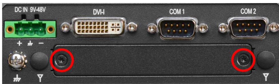
2. Attach the MEC-LAN bracket, and fasten the 2 screws to fix it as indicated.
