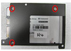
3. Turn over the HDD bracket. Connect the HDD bracket to the SATA connector of the unit and fasten the 3 screws.
