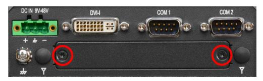
2. Insert CMI-HD module vertically to the female connector on the system's mainboard, and fasten 2 screws to fix it.
