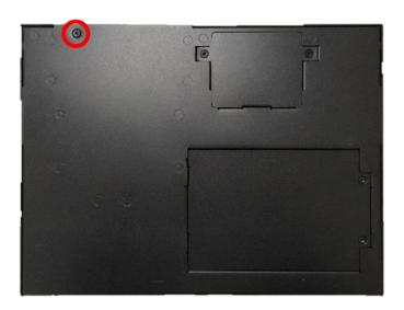
2. Loosen the screw to remove the HDD bay cover bracket.
