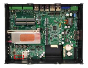
5. Insert the female connector of PoE daughter board to the male connector on system motherboard.
