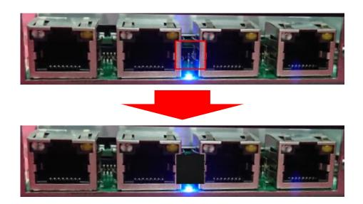
2. Insert the CMI-M12 module vertically into the female connector on system's mainboard until it's connected firmly, and fasten 4 copper pillars to fix it.
