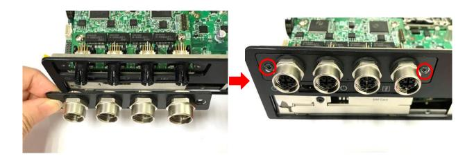
7. Put on the rubber rings to the four M12 LAN ports.
