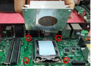
7. Flip the corner of thermal pad and fasten the heatsink with provided 4 screws.
