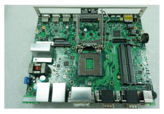
3. Align the notches on CPU with the alignment post on socket.
