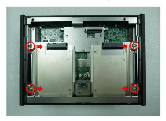
4. Hold front and rear panel and lift up the body of unit vertically.
