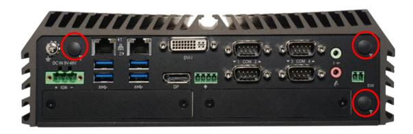
2. Penetrate the antenna jack through the hole at both sides as illustrated.
