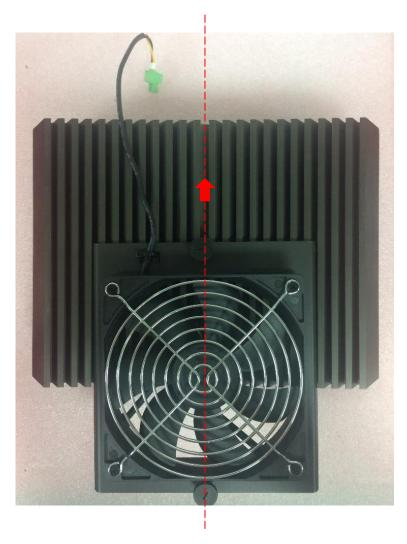
3. Move the fan to the center of chassis. Tighten the 2 screws marked on photo to secure it.
