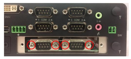
5. Attach the COM bracket. Fasten 2 screws and 4 D-Sub jack screws to fix it..
