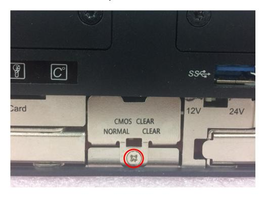
2. Pull out the CMOS battery bracket with assistance of a tweezer.
