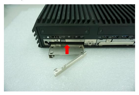
5. Place the rotating arm back and fasten the screw.
