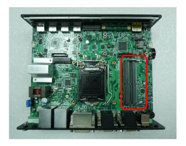
2. Insert a SO-DIMM at a 45-degree angle until its edge connector is connected to SO-DIMM socket firmly.
