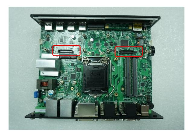
4. Exchange screw to copper pillar before insert the CMI module.
