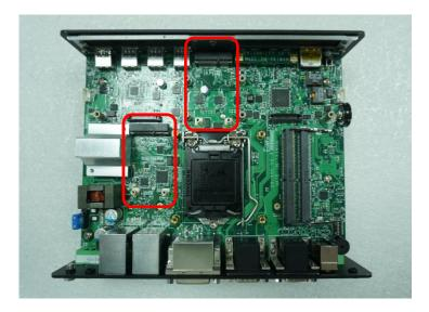
2. Insert the Mini-PCIe card at a 45-degree angle until its edge connector is connected firmly into slot. For 3G/4G Mini-PCIe card, please install on CN3 slot.
