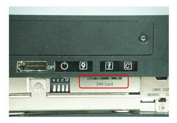
2. Insert a SIM card into SIM slot with the gold contacts facing up. Please pay attention to the insert orientation as illustrated.
