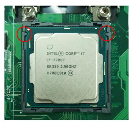
5. Place the thermal pad on the CPU heat spreader. Press down the socket lever to lock the CPU.
