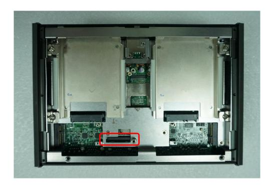
2. Loosen the 2 screws on rear bezel to remove the cover plate.
