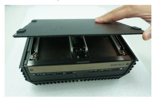
2. Fasten the bottom cover with 6 screws.
