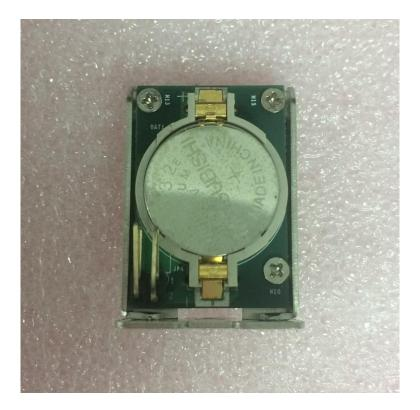
4. Insert the battery bracket firmly and fasten the screw.
