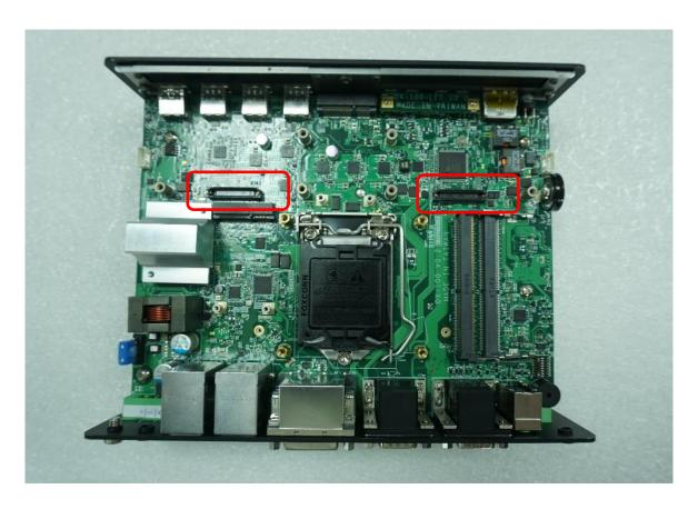
4. Exchange screw to copper pillar before insert the CMI module.
