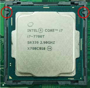
4. The notches of socket provide the space for fingers while lowering the CPU, hold the CPU by the edges toward the notches and insert the CPU gently.
