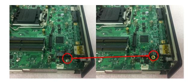
5. Insert the CMI module vertically into the female connector on system's mainboard until it's connected firmly and fasten 4 screws to fix it.
