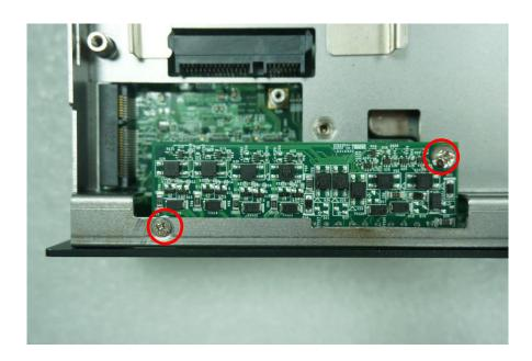
4. Attach the DIO bracket, and fasten 2 screws to fix it.
