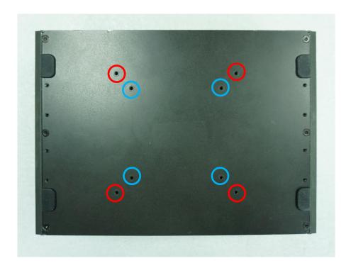
1. The following picture illustrates the installation of DX-1000 series on a VESA stand. Align the 4 screw holes of VESA stand with the screw holes on bottom side of system. Fasten 4 screws to fix it.
