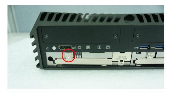
2. Pull the rotating arm and pull the HDD bracket out of system.
