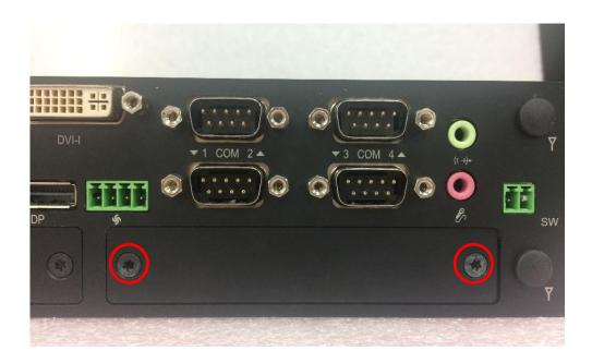
3. Insert the CMI-DIO module carefully into the CMI connector on main board. Fix it with 2 screws.
