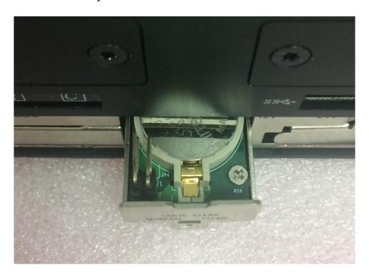
3. Insert a CMOS battery in the battery slot.
