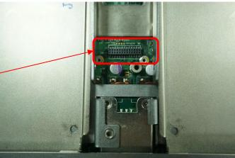
2. Fasten 1 copper pillar before insert IGN module.
