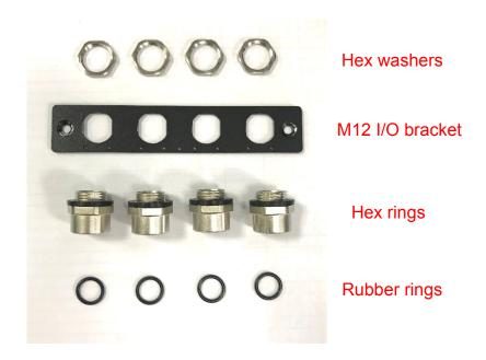
1. Assemble the hex rings, M12 I/O bracket and hex washers together as indicated below: Penetrate hex rings through the M12 I/O bracket holes, and fix them with hex washers.
