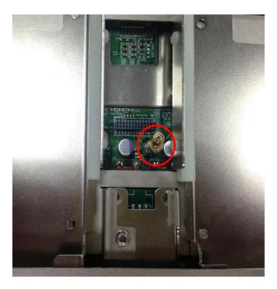
3. Insert IGN module vertically to the female connector on the system's mainboard, and fasten 2 screws to fix it.
