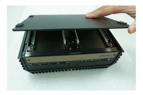
3. Loosen the 4 screws. Pull out 4 latches as marked on photo.
