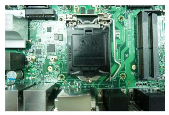
2. Press the CPU socket lever and pull it aside away from the socket to unlock it. Pull back the lever to open the socket.
