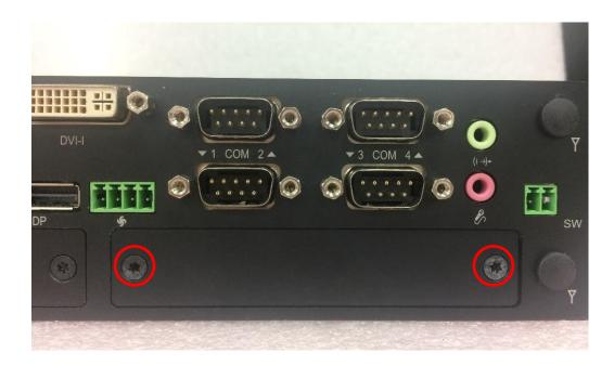
3. Insert the CMI-COM module carefully into the CMI connector on main board. Fix it with 2 screws.
