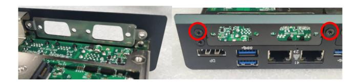
6. Insert the Mini-PCIe card of MEC-COM module at 45-degree angle and insert it to the either slot until the gold-pated connector of module contacted firmly with the slot.
