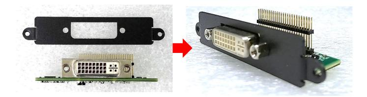
3. Align two holes on the CMI-DVI bracket with the holes on the rear panel.
