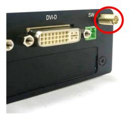
3. Put on washer and fasten the nut with antenna jack.
