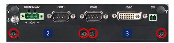
2. Assemble the CMI-COM bracket and CMI-COM module together with 4 D-Sub jack screws
