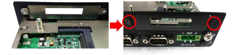
3. Push the connector pins on CMI-DIO module until the pins can be inserted completely to the female connector (BTB\_FH2 or BTB\_FH1) on the system's mainboard.
