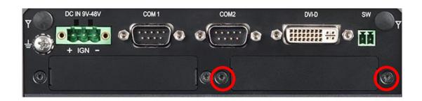
2. Assemble the CMI-DVI bracket and CMI-DVI module together with 2 D-Sub jack screws.
