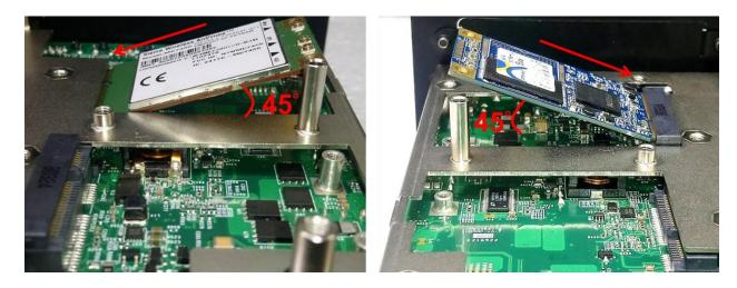
4. Press down the module and fasten two screws to secure the module.
