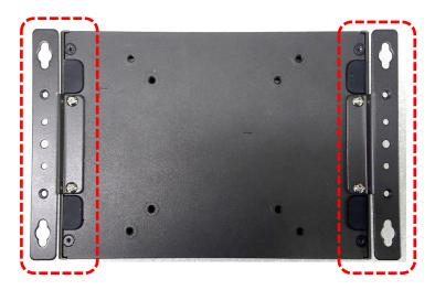
2. Fasten 2 DIN rail mounting clips to mounting brackets on both sides with provided 4 screws as illustrated.
