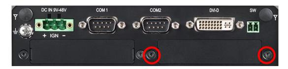
2. Attach the CMI-HD bracket on the backside of system's rear panel, and fasten it with two screws.
