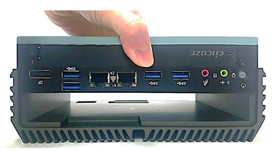
2. Level the grooves on the cover at front and rear panels. Put on the cover.
