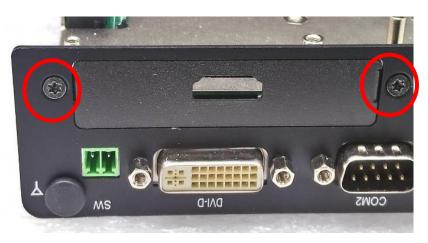
3. Align the hole on CMI-HD module with the screw hole on the system's mainboard module, and insert vertically to the female connector (BTB\_FH1) on the system's mainboard.
