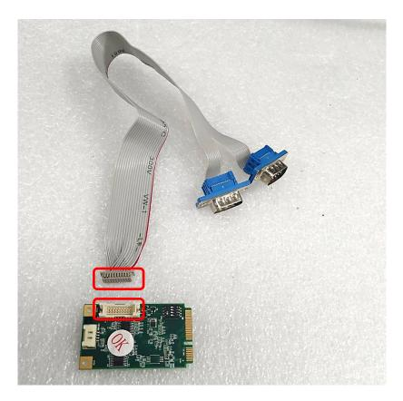
2. Align the protrusion and notch on the two connectors. Insert the female connector on the flat ribbon cable to the connector on MEC-COM module.
