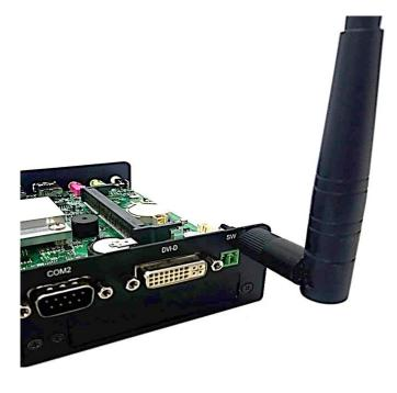
5. Attach the RF connector at another end of cable onto the module.
