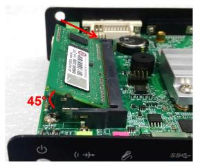
3. Press the modules down until it's fixed firmly by the two locking latches on the sides.
