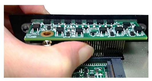
4. Make sure the hole on CMI-DIO module is aligned with the screw hole on the system's mainboard, and fasten a screw to fix it.
