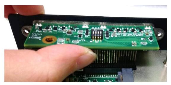
5. Make sure the hole on CMI-COM module is aligned with the screw hole on the system's mainboard, and fasten a screw to fix it.
