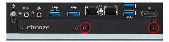
5. Attach the MEC-COM bracket on the back side of system's front panel, and fasten it with two screws.
