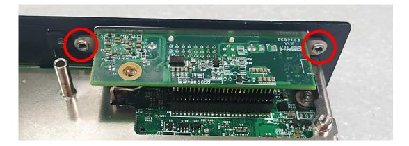
4. Push the connector pins on CMI-DVI module until the pins can be inserted completely to the female connector (BTB\_FH1) on the system's mainboard.
