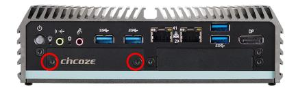
2. SIM card slots are at the front panel of the system.
