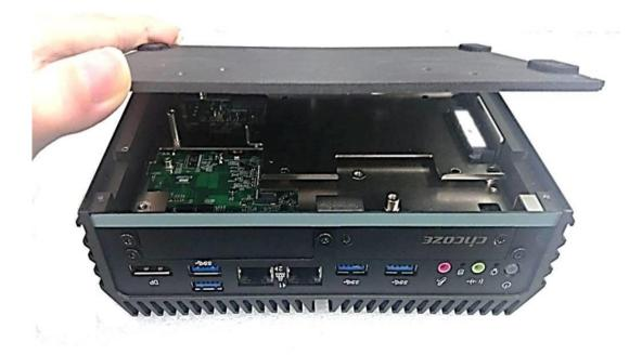
3. Fasten the 4 screws to fix the cover.
