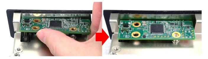
2. Fasten a screw to fix the CFM-IGN Module.
