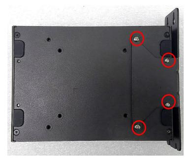
3. It is achievable to mount system on the wall by fastening the screws through the bracket mounting hole.
