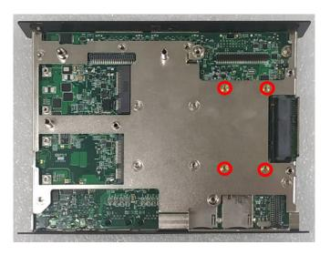
3. Connect the Half Slim SSD to the SATA connector and fasten the 4 screws.
