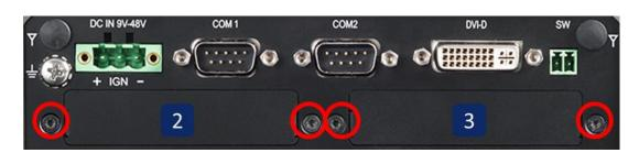
2. Attach the CMI-DIO bracket on the backside of system's rear panel, and fasten it with two screws.
