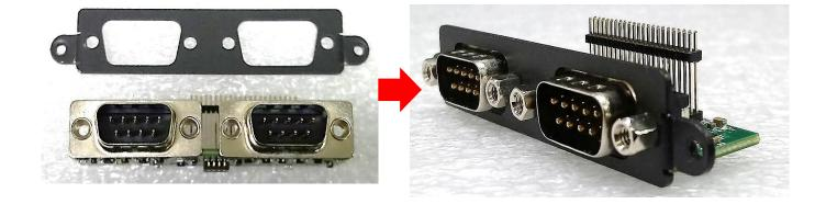
3. Align two holes on the CMI-COM bracket with the holes on the rear panel.
