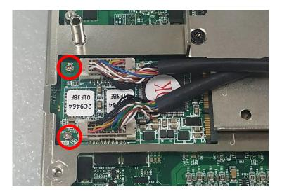
6. Attach the LAN board of MEC-LAN module onto bracket from the back side.
