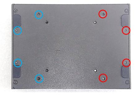
2. Place the side mount bracket on the bottom of system as shown in the picture below, and fasten the rest of 4 screws to fix the side mount bracket with system together.
