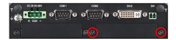
2. Assemble the CMI-VGA bracket and CMI-VGA module together with 2 D-Sub jack screws.
