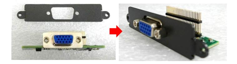
3. Align two holes on the CMI-VGA bracket with the holes on the rear panel.
