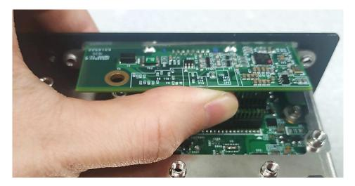
5. Align the screw hole on CMI-VGA module with the screw hole on the system's mainboard, and fasten a screw to fix it.
