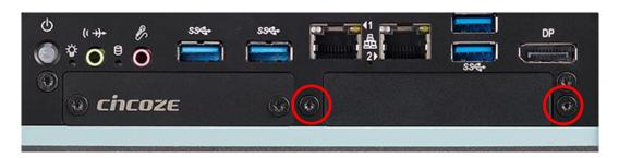
3. Attach the MEC-LAN bracket on the back side of system's front panel, and fasten it with two screws.
