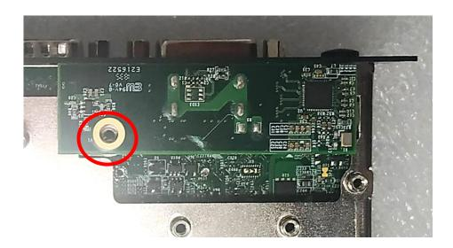
4. Fasten a screw to fix the CMI-HD module.
