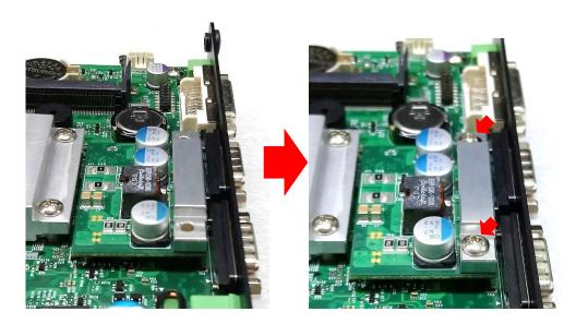
4. Paste the thermal pads onto the heatsink and coil carefully.
