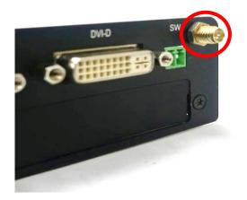
4. Assemble the antenna and antenna jack together.
