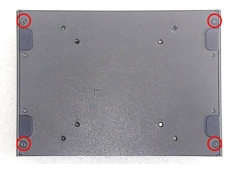
2. Remove the bottom cover from the chassis.
