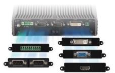
Flexible & Modular Design Based on Cincoze' exclusive CMI (Combined Multiple I/O) and CFM (Control Function Module) technologies, the DC-1200 can be easily configured to increase specified functions and a variety of I/O modules.
