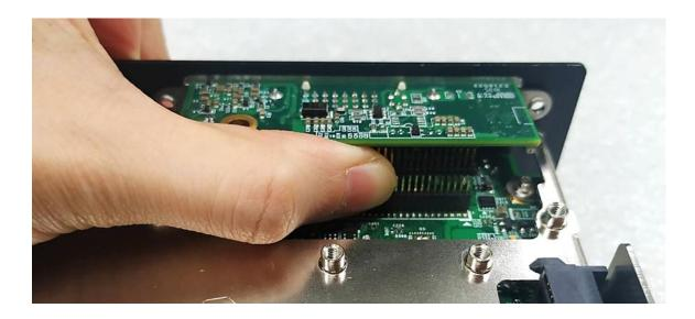
5. Align the hole on CMI-DVI module with the screw hole on the system's mainboard, and fasten a screw to fix it.
