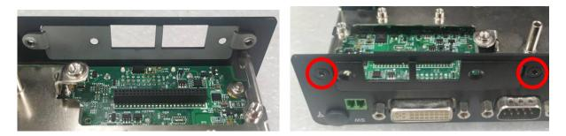
4. Insert the Mini-PCIe card of MEC-LAN module at 45-degree angle and insert it to the either slot until the gold-pated connector of module contacted firmly with the slot.
