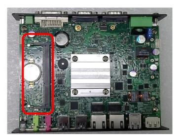
2. Tilt the SO-DIMM module at a 45-degree angle and insert it to SO-DIMM socket until the gold-pated connector of module contacted firmly with the socket.
