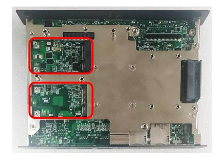
2. Unscrew the 2 screws to remove bracket#1 from the front panel.
