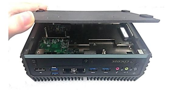
3. Hold front and rear panel and lift up the body of unit vertically.
