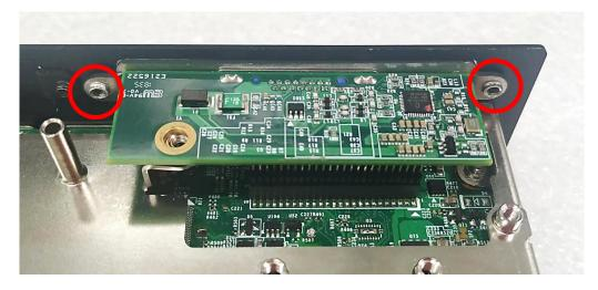
4. Push the connector pins on CMI-VGA module until the pins can be inserted completely to the female connector (BTB\_FH1) on the system's mainboard.
