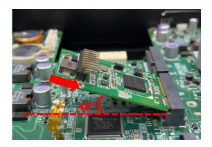
Step 4. Press the card down and secure it with 2 screws.
