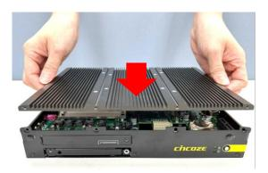
Step 2. Fasten the eight screws at front and rear panel to secure the top cover.
