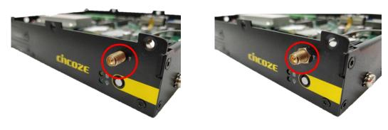
Step 3. Assemble the antenna and antenna jack together.
