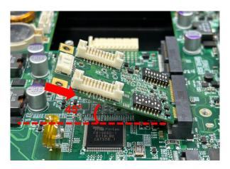
Step 4. Press the card down and secure it with 2 screws.
