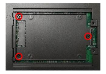
Step 4. Place the HDD bracket on screw-hole side of HDD. Use four screws provided to assemble HDD on the bracket.
