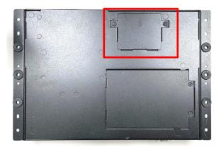
Step 2. Loosen two screws to remove the cover.
