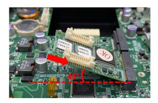
Step 4. Press the card down and secure it with 2 screws.
