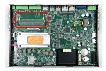
Step 2. Tilt the memory module at a 45-degree angle, and insert it into SO-DIMM socket until the golden finger connector of the module is seated firmly.
