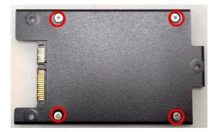
Step 5. Seat the HDD bracket into HDD compartment, and line up the connector of HDD with SATA slot, then push it until HDD is fully connected into slot.
