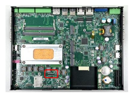
Step 2. Insert the female connector of power ignition board to the male connector on system motherboard.
