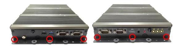
Step 4. Attach the P2202 to wall by fastening screws through mounting holes at each side as illustrated.
