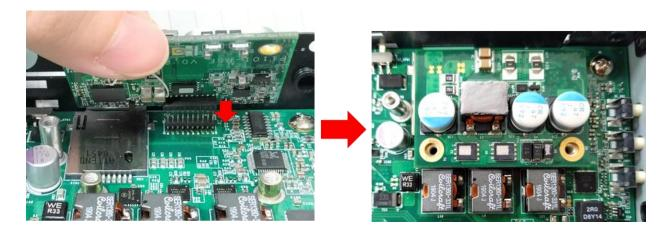
Step 6. Put on the PoE thermal block and fasten two screws to secure the PoE board.
