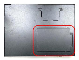
Step 2. Loosen the two screws, lift the cover, and then remove it.
