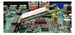
Step 4. Press down the card and secure it with two screws.
