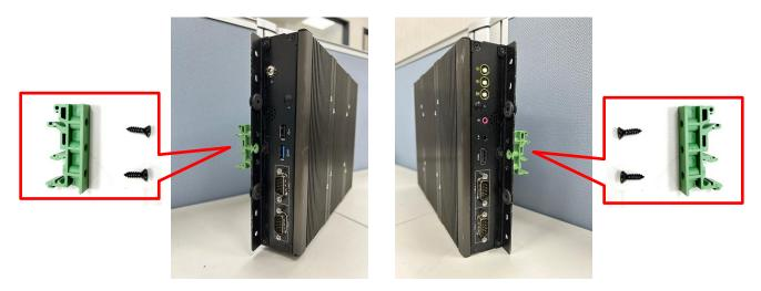
Step 3. Clip the system into DIN rail as illustrated by the following steps. (1) Have upper end of mounting clip snaps into the DIN rail. (2) Press the system toward to have lower end of mounting clip snaps into the other side of DIN rail.
