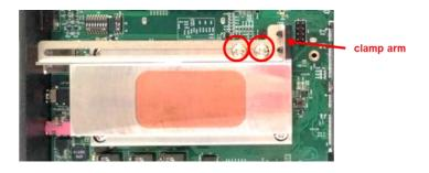
Step 8. Slide the clamp arm of retention module until it contacts the edge of PCI(e) expansion card.
