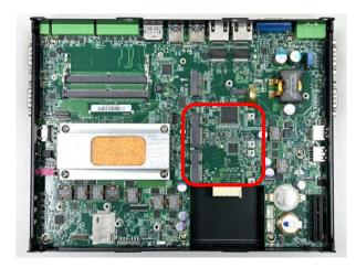
Step 3. Tilt the Mini PCIe card at a 45-degree angle and insert it to the socket until the golden finger connector of the card seated firmly.
