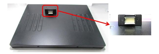
Step 4. Place the P2202 on the display module through its display connector hole as indicated.
