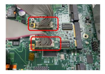
Step 7. Attach the COM ports onto the back side of the cover plates, and then fasten the 8 D-Sub jack screws to secure the COM ports.
