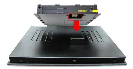
Step 5. Align the mounting holes of P2202 with the screw holes of display module underneath. Slide the P2202 until it and the display module connected together, and then fasten six screws to secure P2202 on the display module.
