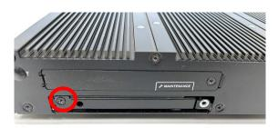
Step 8. Put back HDD bay cover at front panel, and fasten it with the screw.
