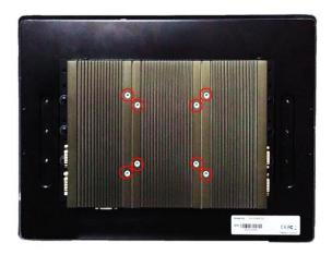
Step 1. The following picture uses a panel PC (P2202+ Display Module) as a demonstration. To attach the panel PC to a VESA stand, please fasten eight screws as indicated to fix it on the stand. (Please refer to section 3.13 in this manual for how to connect P2202 with a display module.)
