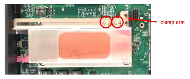
9. Slide the clamp arm of retention module until it contacts the edge of PCI(e) expansion card.
