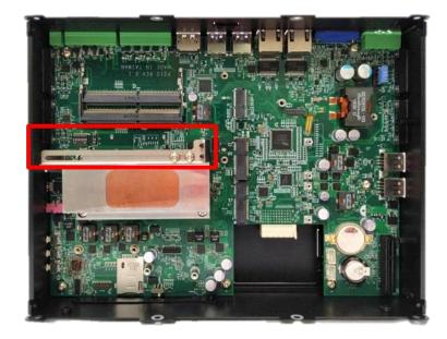
8. Loosen the two screw as indicated to have the clamp arm slidable.
