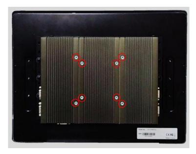
1. The following picture uses a panel PC (P2102+CV display module) as a demonstration. To attach the panel PC to a VESA stand, please fasten eight screws as indicated to fix it on the stand. (Please refer to section 3.13 in this manual for how to attach PC2102 to CV/CS display module.)
