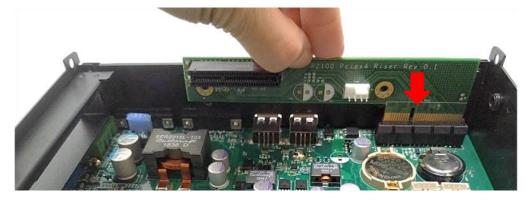
5. Align the notch of golden fingers of PCI(e) card with the expansion slot. Insert the card horizontally, and press the card straight down into the slot until it's seated firmly.
