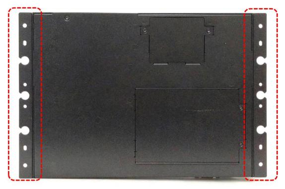
2. Fasten 2 DIN rail mounting clips to mounting brackets on both sides with provided 4 screws (with each screw size of T3x10.5) as illustrated.
