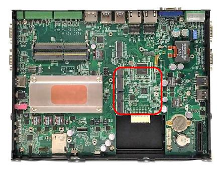
2. Tilt the Mini PCIe card at a 45-degree angle and insert it to the socket until the golden finger connector of the card seated firmly.
