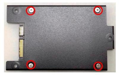
5. Seat the HDD bracket into HDD compartment, and line up the connector of HDD with SATA slot, then push it until HDD is fully connected into slot.
