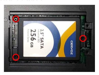
7. Put back the cover and fasten the two screws.
