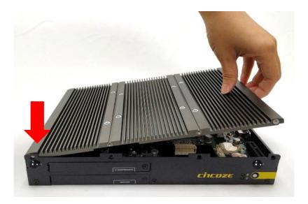
2. Fasten the eight screws at front and rear panel to secure the top cover.
