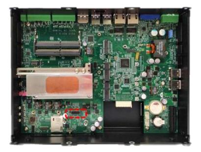
2. Insert the female connector of power ignition board to the male connector on system motherboard.
