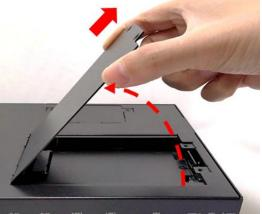
3. Loosen three screws and take the HDD bracket out of HDD compartment.
