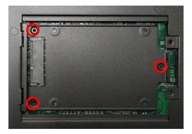
4. Place the HDD bracket on screw-hole side of HDD. Use four screws provided to assemble HDD on the bracket.
