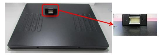
6. Place the P2102 on the display module through its display connector hole as indicated.
