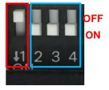
Default setting of Pin1 to Pin4 is OFF/ON/ON/ON.
